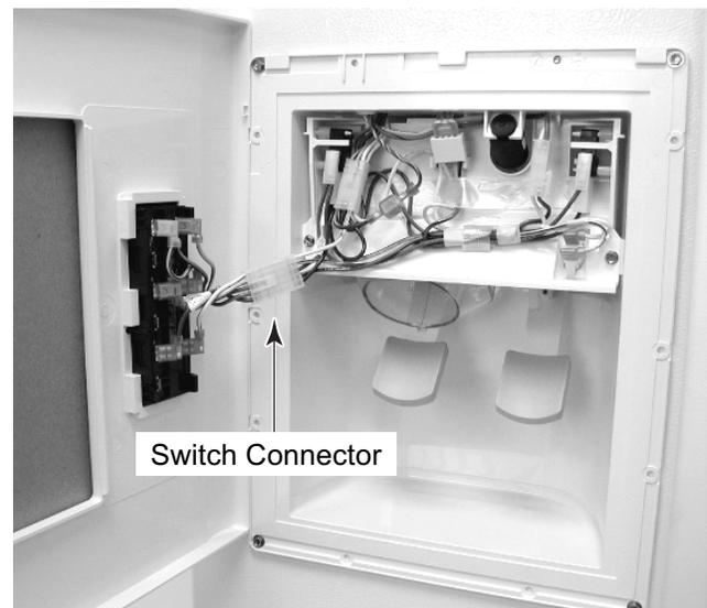
5. Disconnect the three wire connectors and the green ground wire from the switch subpanel.
