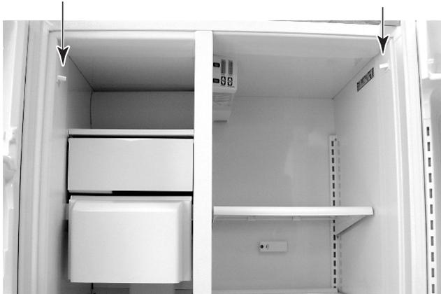
3. Use a small-bladed screwdriver and pry the door switch out of the freezer/refrigerator liner opening.
