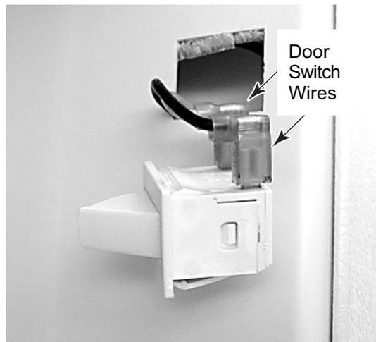
**REASSEMBLY NOTE:** Be sure to position either door switch with the straight side facing the front (see the top photo) before you press it into the opening.
