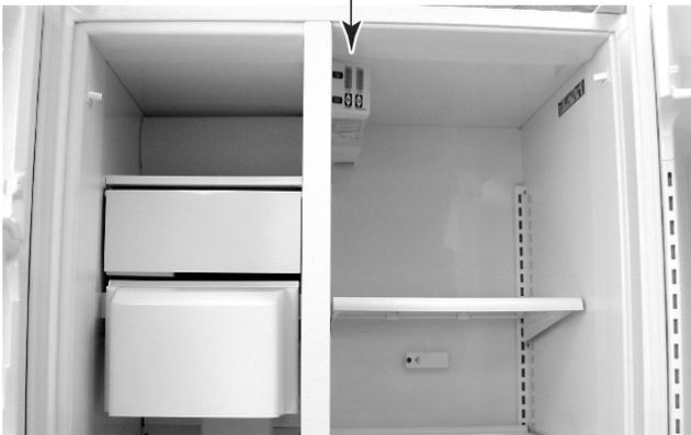
3. Remove the light shield. To do this, place your finger into the half-moon slot at the bottom of the shield and pull out, then pull down to disengage the corners from the control box.
