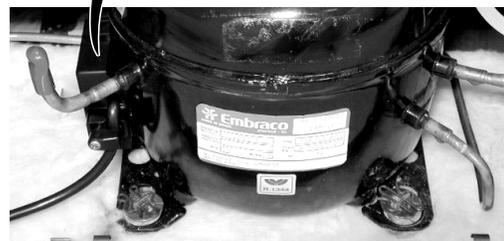
8. Access the sealed system and discharge the refrigerant into an approved recovery system.
