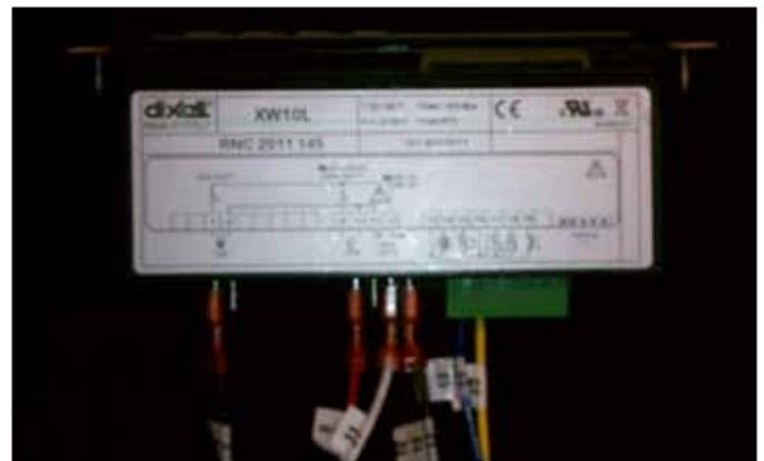
4. Slide the controller back into the cabinet / housing and re-fasten securely with the previously used method.
