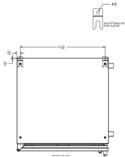
Use the above illustrations to locate the holes needed for your specific model. Mount the brackets as shown in Illustrations 2A and 2B, then slide the cabinet into the opening to engage and prevent tip during use.
