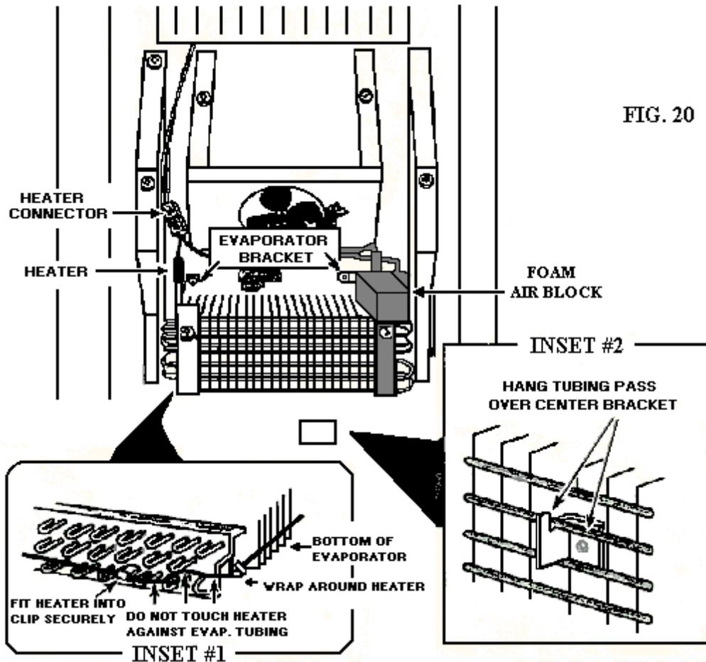
1. Remove the foam air-block at the upper right corner of the evaporator from around the evaporator tubing.
