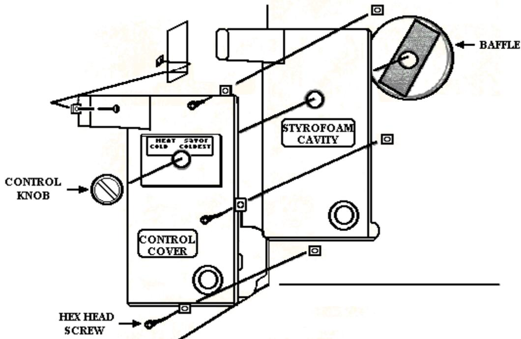
1. Remove the four hex head screws securing the meat savor control to the cabinet liner.
