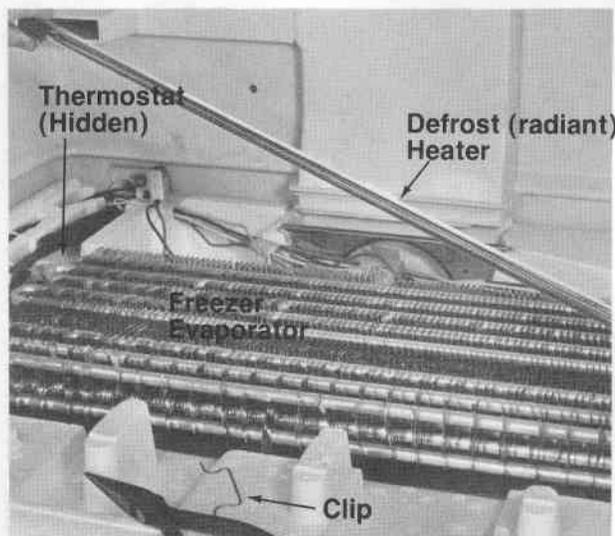
An ohmmeter check will determine if all phases of the defrost cycle are functioning properly. The defrost thermostat contacts open at approximately  $+47^{\circ}\text{F}$  and close at approximately  $+15^{\circ}\text{F}$ .
