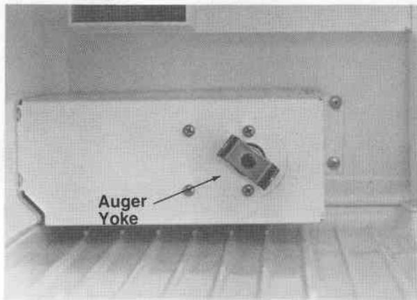
The auger motor is located behind the ice storage bin. The yoke fastened to the motor engages the drive ring and turns auger in a clockwise direction. Both the yoke and drive ring are designed to prevent a loosening of the yoke by exerting counter pressure while in operation.
