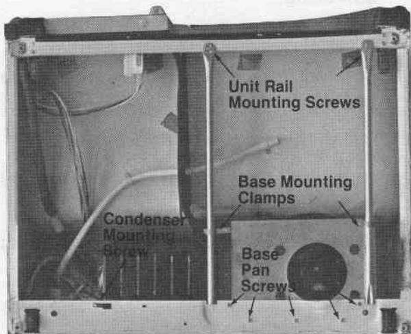
4. Remove the rear mounting screw from the air divider baffle.
