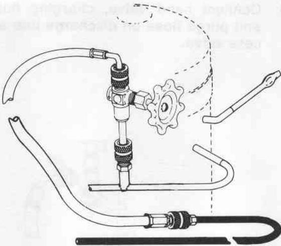
6. Slowly open hand valve and discharge system for 5 minutes, with compressor not running.
