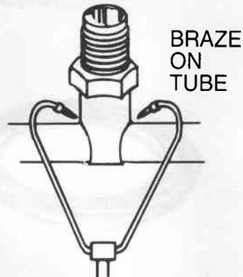
3. Leak check permanent access valve with refrigerant gas from top valve of charging cylinder connected through charging hose and hand valve to access valve (Step 4).
