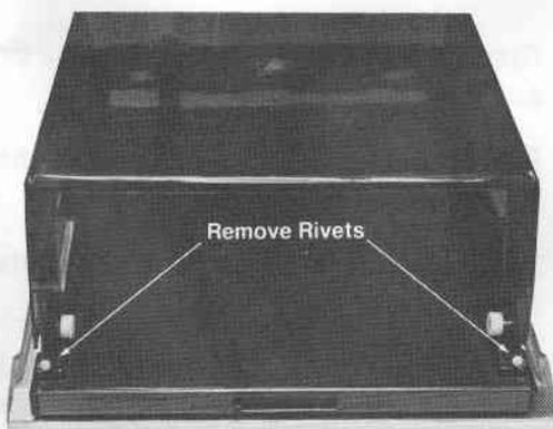
4. Lift the front of the drawer and pull it out of the shelf frame.
