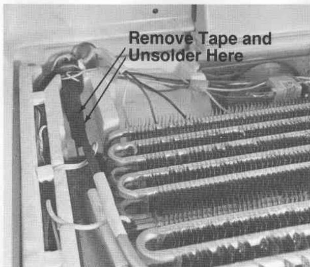
17. Transfer the rubber sleeve to the replacement heat exchanger and tape both ends.
