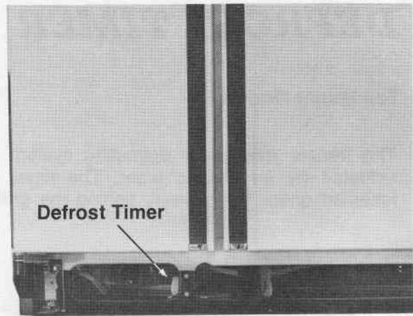
The timer control shaft is designed for screwdriver adjustment. When manually setting the timer to initiate defrosting, turn the control shaft clockwise until you establish the approximate location of the defrost cycle. Then turn the shaft slowly and stop immediately when the first click is heard.
