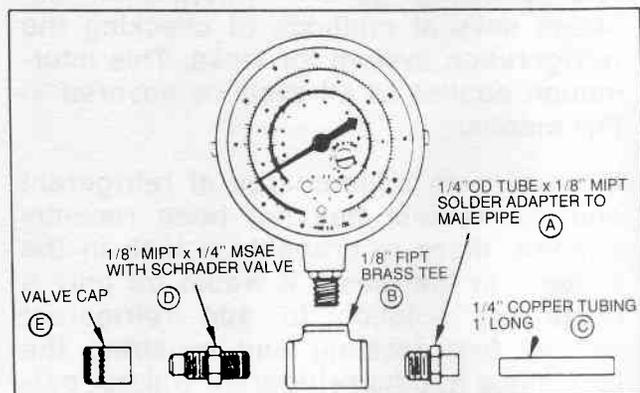
4. Apply 200 lbs. pressure at the Schrader valve and leak test the access fitting with a soap solution.
