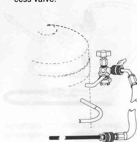
7. Connect purge hose to the temporary piercing valve on compressor process stub.
