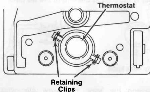
Using needle nose pliers, grasp one of the thermostat clips and pull out. Press in new thermostat, making sure that pins are properly indexed. Using this procedure, it is not necessary to remove the electrical assembly. If you are replacing the module, transfer the clips to the new mold support. (Use new thermal bonding material.)
