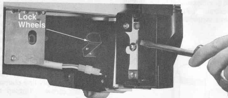
If the floor is not level and it is necessary to raise the rear of the cabinet, we suggest rolling the rear wheels on to a piece of plywood or other shim material.
