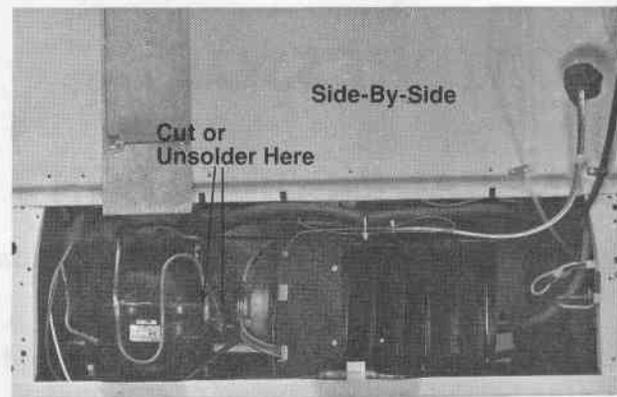
5. Disconnect the lead wires from the compressor terminals.
