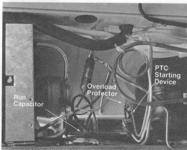
The PTC solid state starting device is a push-on component mounted to the start
