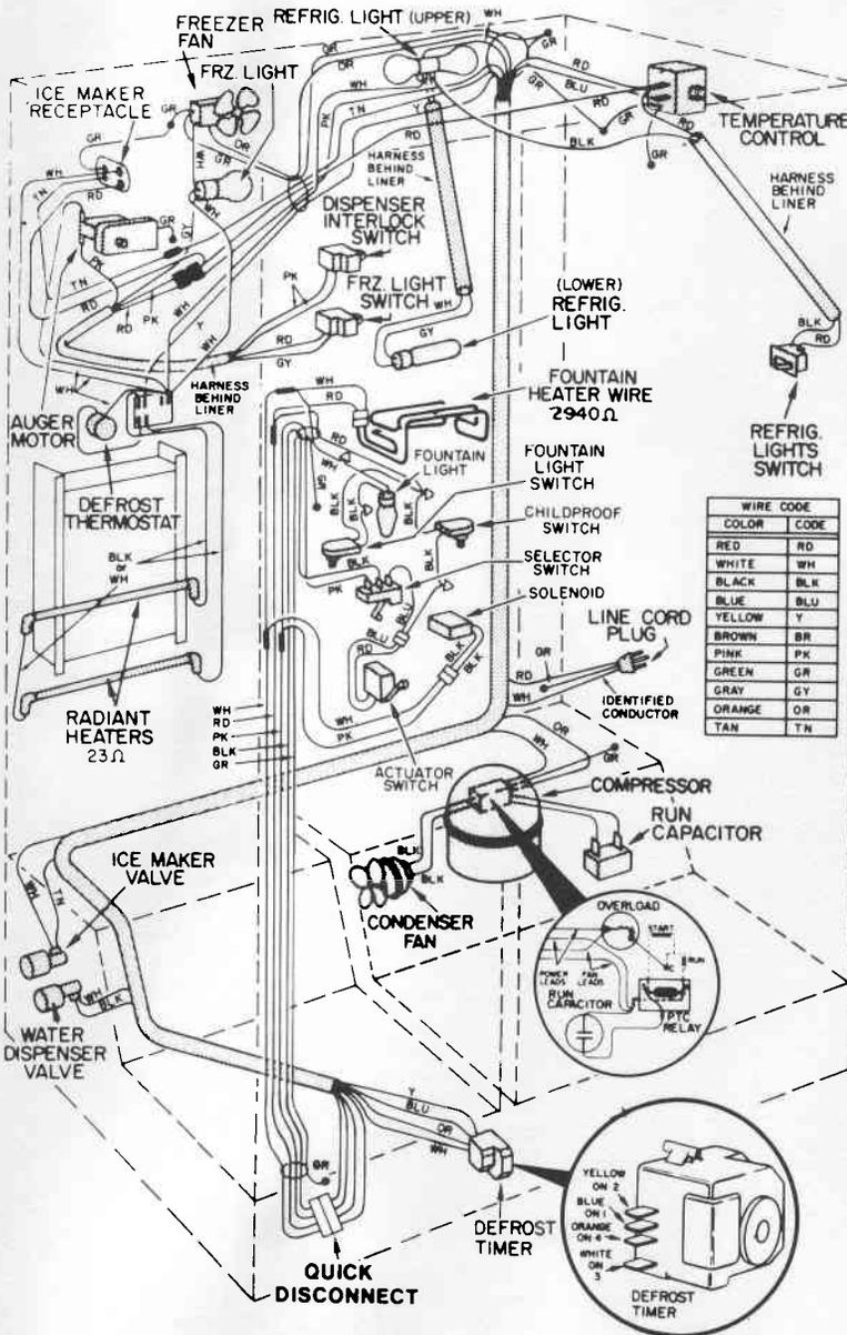
**SCHEMATIC WIRING DIAGRAM**
