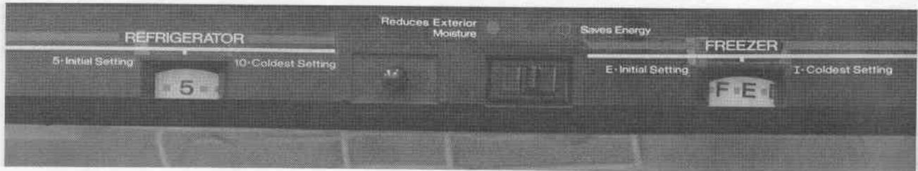
These models have two temperature controls: fresh food and freezer compartment. The fresh food temperature control senses the temperature of its compartment and governs the compressor operation accordingly. The freezer compartment control adjusts a baffle which regulates the amount of air allowed to enter the fresh food compartment.
