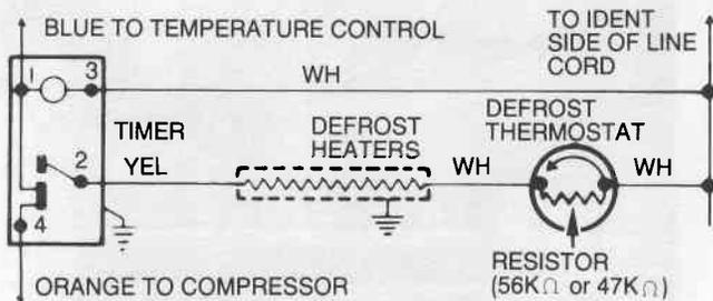
If there is no resistance reading (open circuit) the defrost heater and thermostat must be checked individually. **NOTE:** When using the meter avoid touching the probes since this could result in a false reading and misdiagnosis.
