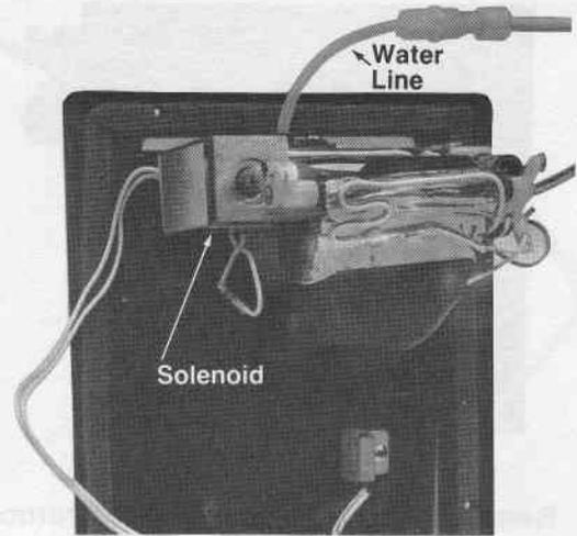
**NOTE:** To check trap door for ice chute, activate solenoid by using switch on dispenser.
