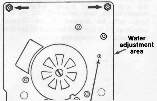
When small hole is centered in larger hole the water fill adjustment is for 7.5 seconds fill time (normal).
