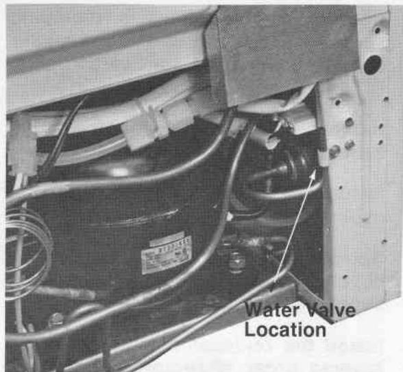
4. Disconnect the water inlet fitting from the water valve and drain the water into a container.
