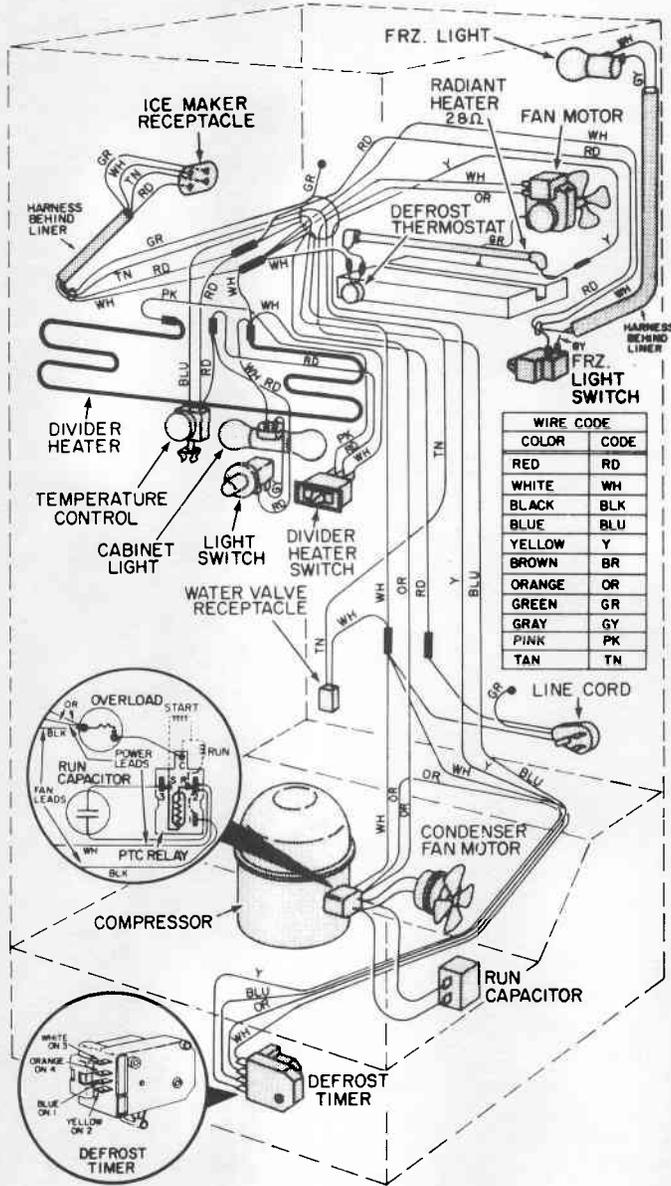
**SCHEMATIC WIRING DIAGRAM**
