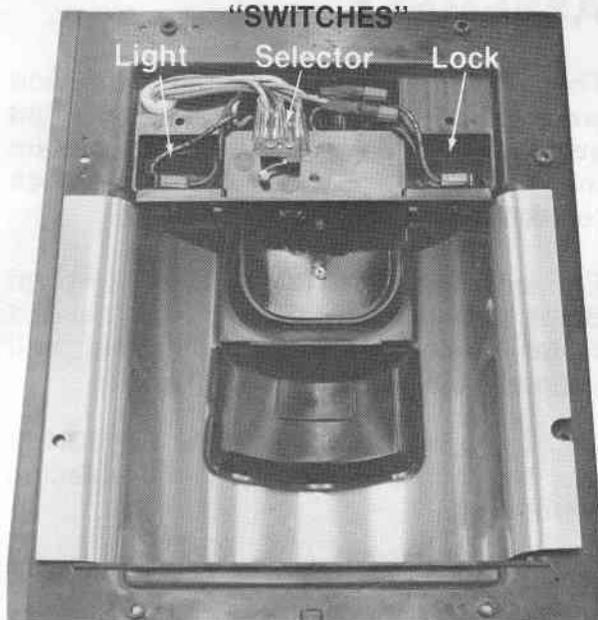
6. Remove screw from side of fountain that will allow removal of well trim. Carefully pull the trim out of the fountain so you do not damage it.
