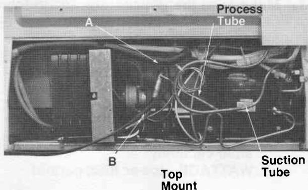
4. Crimp and solder the yoder tubing at point "A".
