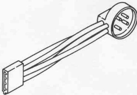
This harness plugs directly into liner receptacle.
