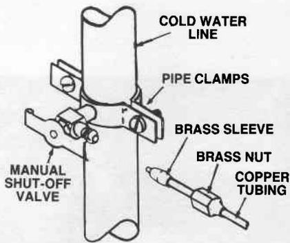
5. Turn ON the main water supply and flush out the water pipe until water runs clear. At the same time, check for leaks at the saddle valve. After the water has cleared, flush out the tubing from the saddle valve to the water valve into a bucket by turning the saddle valve on. When the water has cleared, turn off the saddle valve.
