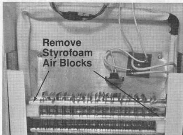
These blocks must be reinstalled the same way as they were before removal.
