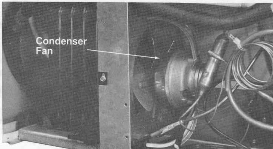
The condenser fan is connected in parallel with the compressor. If the compressor runs but the fan doesn't, the fan is either defective or disconnected. If neither operates, check the cold control, defrost timer, and the cabinet wiring.
