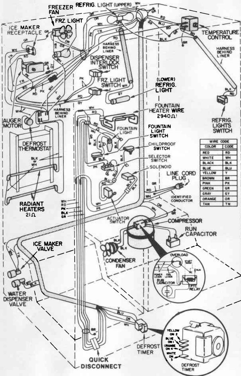
**SCHEMATIC WIRING DIAGRAM**
