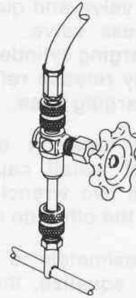
12. Attach hand valve to access valve. Charge in 4 oz. of refrigerant for leak check. Close hand valve. Wait approximately 5 minutes for pressure to equalize. (Leak check low side).
