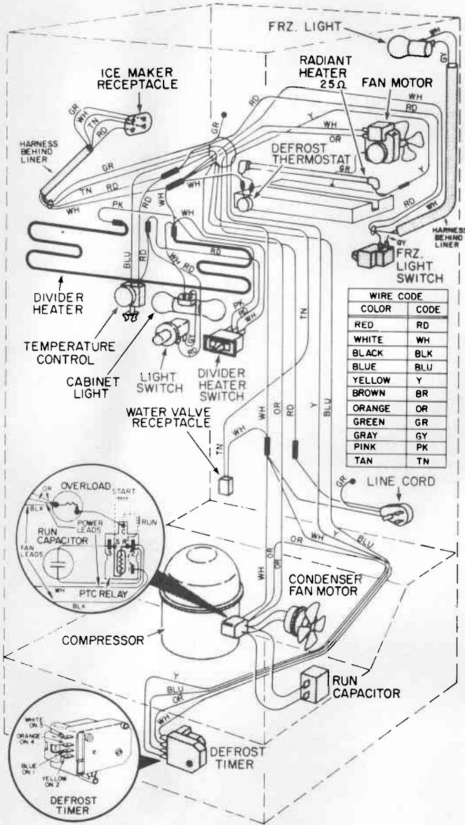
**SCHEMATIC WIRING DIAGRAM**
