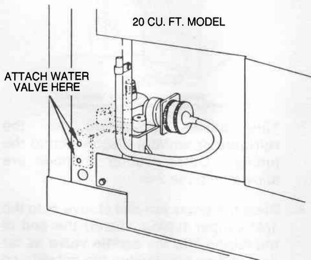
3. Locate water valve power plug and water line inside machine compartment. Remove protective cap from water line and discard. Slip the plastic nut on water line.
