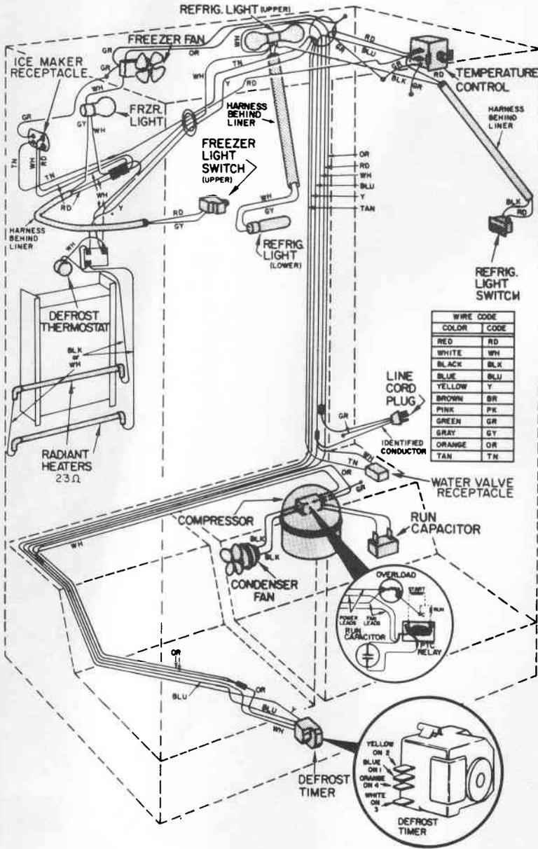
**SCHEMATIC WIRING DIAGRAM**
