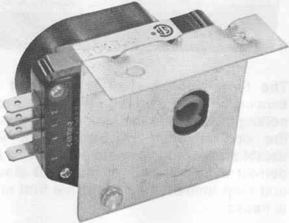
The timer control shaft is designed for screwdriver adjustment. When manually setting the timer to initiate defrosting, turn the control shaft clockwise until you establish the approximate location of the defrost cycle. Then turn the shaft slowly and stop immediately when the first click is heard. The schematic illustrates the timer circuits in sequence.
