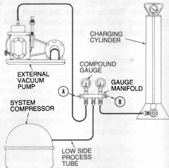
6. Close the manifold valve "A" and stop the vacuum pump.
