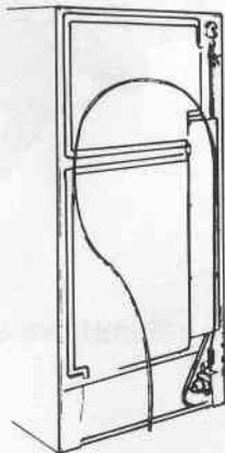
This allows movement for the refrigerator without disconnecting the tubing. Other routing methods are shown on page 2-8.
