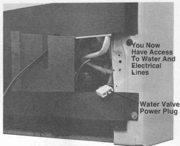
3. Fit the plastic tubing into the water valve as far as it will go and tighten the compression nut, finger tight. Then with a wrench, tighten the nut 3/4 of a turn.
