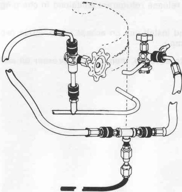
9. Slowly open hand valve and temporary piercing valve and discharge system for at least five minutes or until refrigerant is completely released.
