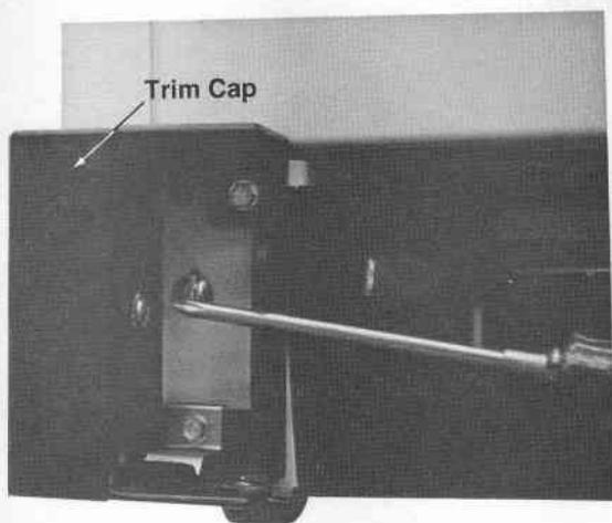
21. Remove bottom hinge using a Torx-T27 drive and move to the opposite side of cabinet and reinstall using the same screws.
