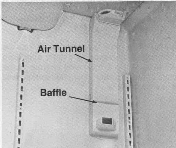
air flow to the freezer compartment which, therefore, further lowers the temperature of the freezer compartment.
