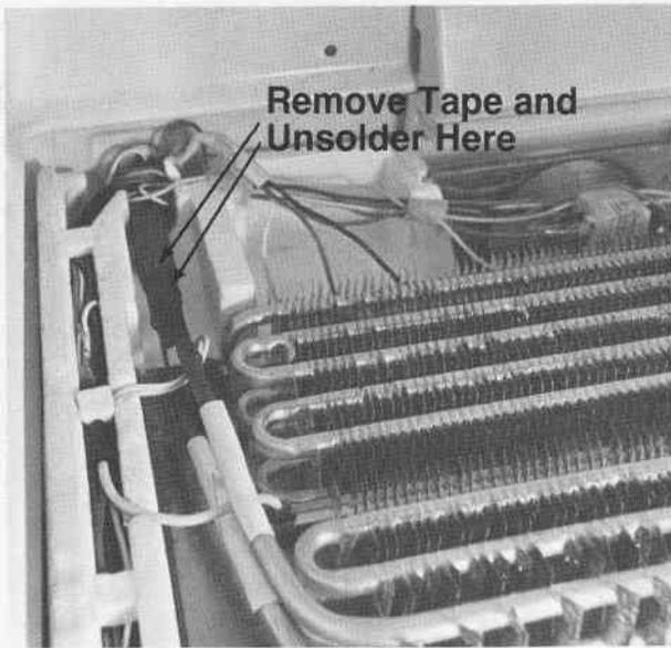
19. Visually check the soldered joints for leaks.
