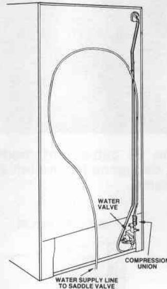
Supply Line Connection to Water Valve
