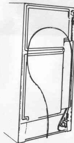
5. Locate the brass nut and sleeve which come with the saddle valve. Slide them onto the 1/4" copper tubing. Insert the end of the tubing into the saddle valve as far as it will go and tighten the nut with an adjustable wrench. Turn off the saddle valve.
