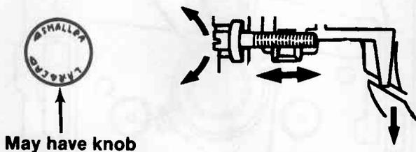
Turning the knob or screw clockwise decreases fill; counterclockwise increases the fill amount.
