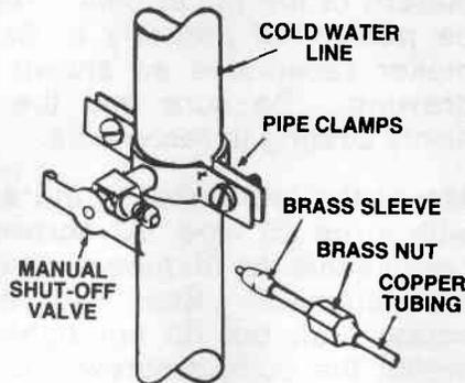
6. Turn ON the main water supply and flush out the tubing until the water runs clear. At the same time, check for leaks at the saddle valve. Next, prepare to flush out the 1/4" tubing. Position a bucket or other container at the open end of the 1/4" tubing so it will catch the water. Turn on the saddle valve and allow water to flow until it has cleared. Turn off saddle valve.
