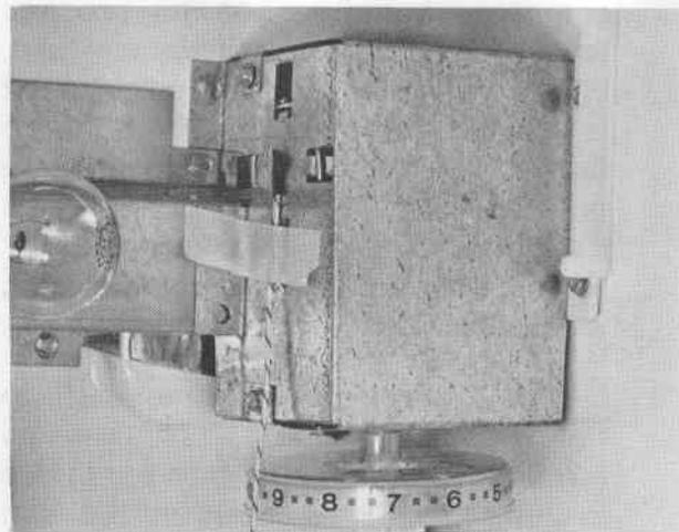
The cut-in temperature will be approximately 1-2 degrees higher than the specified temperatures.
