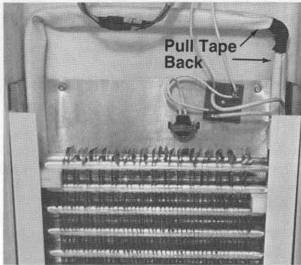
15. Unsolder the heat exchanger tubing at the points as indicated. This will free the old heat exchanger.
