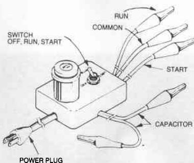
The tester leads are marked RUN, START, and COMMON. Connect the common lead to the common terminal of the compressor, the start lead to the start terminal and the run lead to the run terminal. The compressor terminal arrangements are illustrated below. The
