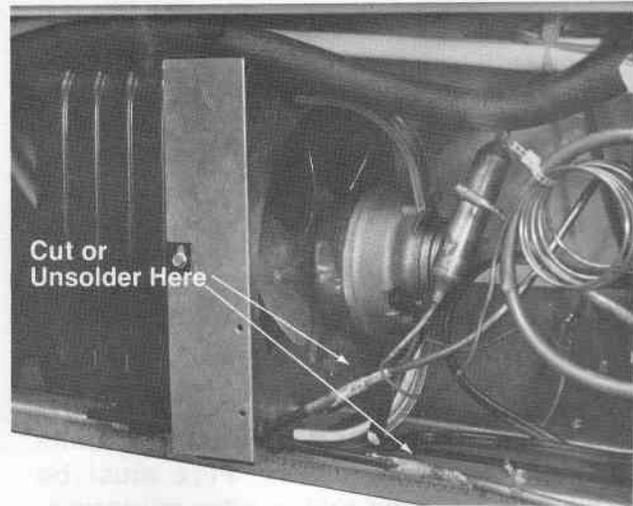
10. Remove the condenser screws.
