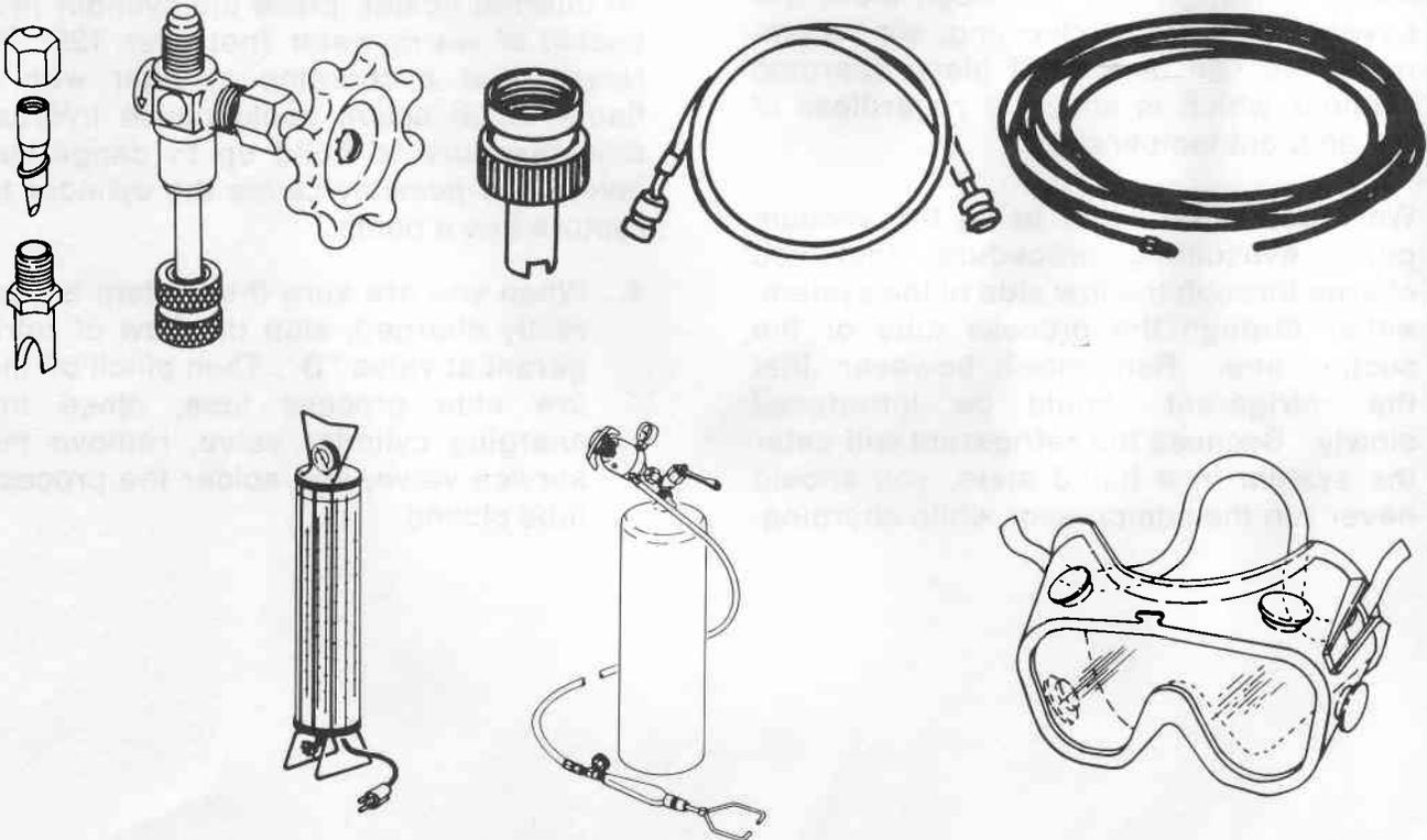
**NOTE:** Always use a purge hose of sufficient length to discharge the refrigerant out of the work area - preferably out doors. Keep work area well ventilated when purging or discharging refrigerant. **WEAR GOGGLES TO PREVENT EYE INJURY** when handling refrigerant.
