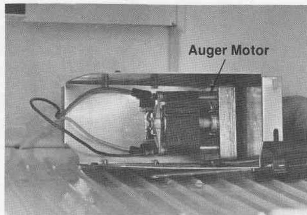
The auger motor is easily be removed:
