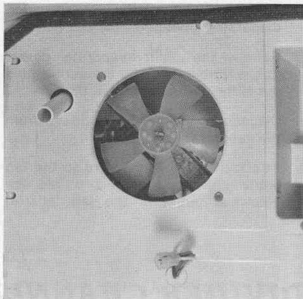
The freezer fan is designed to draw air up from the bottom of the freezer compartment; pull it through the coil area and blow it out at the top against a dispersing shield, thus creating a pressure chamber behind the shield. From here the air is dispersed in three directions. The fan is wired to run simultaneously with the compressor.
