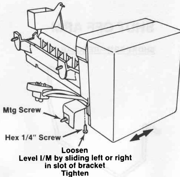
Make sure refrigerator is level front to back (Adjust legs or rollers.)
