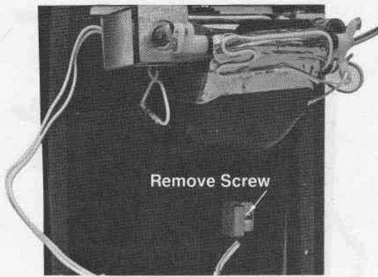
3. Remove two (2) screws to remove switch from bracket.
