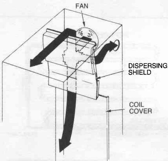
Because the evaporator is the coldest surface in the freezer, all moisture in the compartment forms on its surfaces. After eight hours of accumulated compressor running time, the evaporator is automatically defrosted and the water drains into a tray in the machine compartment.
