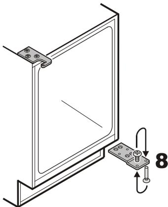
8. Transfer both pins of the hinge plate to the opposite side.
