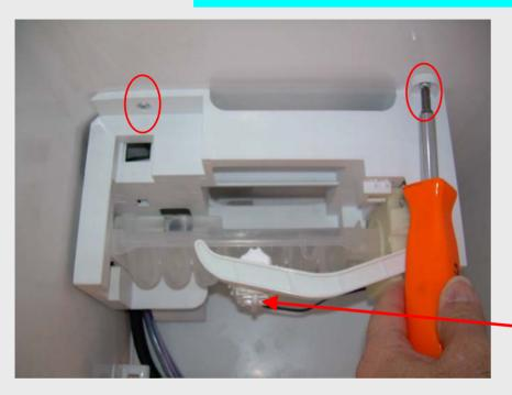
Remove screws then pull icemaker forward off of rear support.
