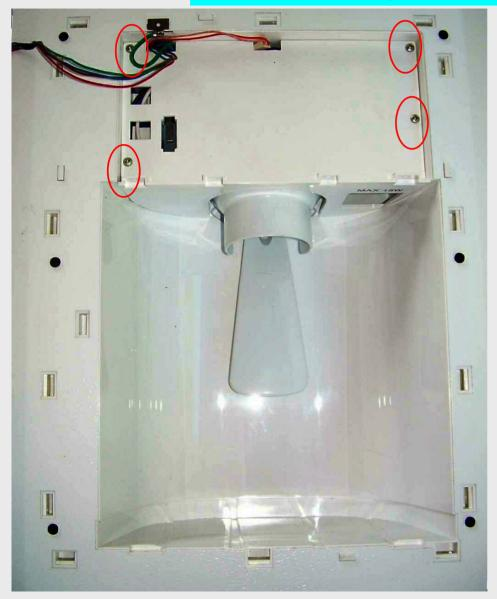
Remove screws (4) and pull paddle assembly outward to access paddle, dispenser door and solenoid.
