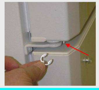
Door height is adjusted by adding shims under each door.
