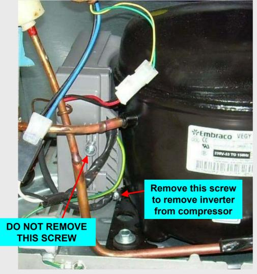
To remove inverter remove 1 screw and pull inverter box upward and to the left
