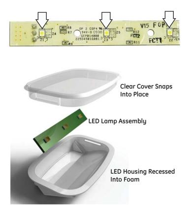
The LED boards are all wired in a parallel circuit and operate simultaneously. There is a momentary delay in brightness as the LEDs come on. This is normal.
