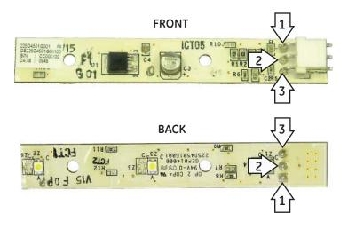
The LED board is defective if both DC voltages are present and the LEDs are not lighting. These boards can also be swapped for testing.
