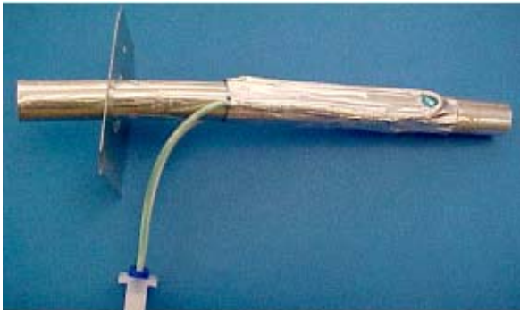
Figure 1 – Assemble grounding plate to tube end with heater electrical connector.
