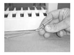
2) Continue to slide the extension arm down the feeler arm through the second loop. Continue to slide all the way forward.
