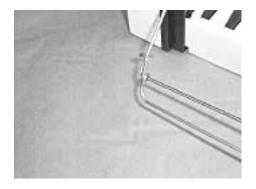
**3)** Once the extension arm is all the way forward, rotate the "hook" end until it engages the vertical portion of the feeler arm.
