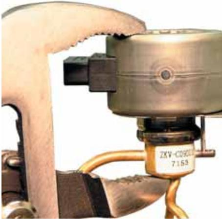
11. Remove the old drier by unbrazing or cutting the condenser loop (halo) as close as possible to the drier. Install the new drier assembly (part # WR86X93).
