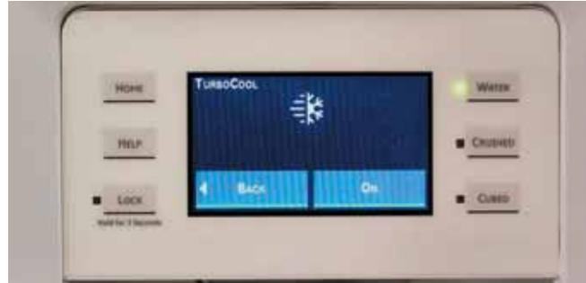
**Note:** The refrigerator temperature cannot be changed during **TurboCool**. The freezer temperature is not affected during **TurboCool**. When opening the refrigerator door during **TurboCool**, the fans will continue to run if they have cycled on.
