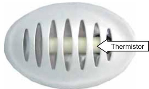
If both freezer and fresh food thermistors are satisfied, the compressor cycles off. If the freezer still requires cooling, the main control board rotates the 3-way valve to stop refrigerant flow to the fresh food evaporator. Even though refrigerant flow has stopped in the fresh food evaporator, the fresh food fan continues to run at low speed.
