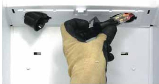
**Note:** The evaporator cover is held in place by four ¼-in. hex-head screws and 2 top tabs. The tabs are inserted into recessed slots in the bottom of the evaporator fan plenum.
