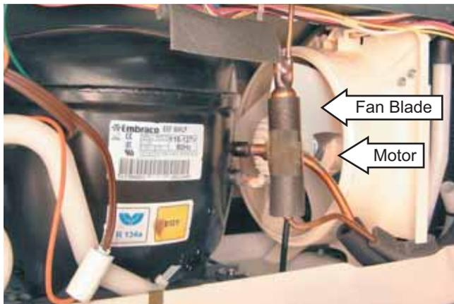
On inverter compressor models, condenser fan speed coincides with compressor speed (low, medium, high) to minimize pressure variations in the sealed system except when the freezer temperature is 20°F above the set point. If this condition exists (such as during initial startup), the condenser fan operates at super high speed while the compressor operates at medium speed.
