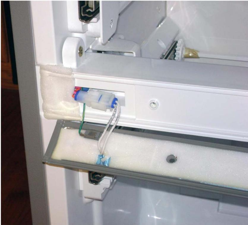
Remove 4 screws securing mullion heater and face plate.
