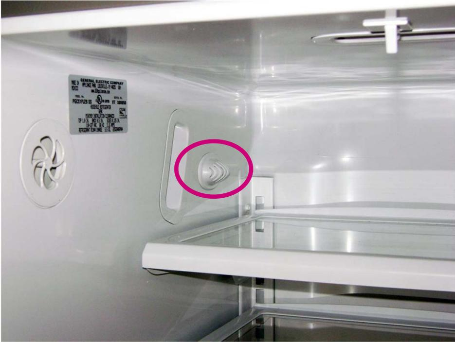
FF Thermistor located on top left side wall
