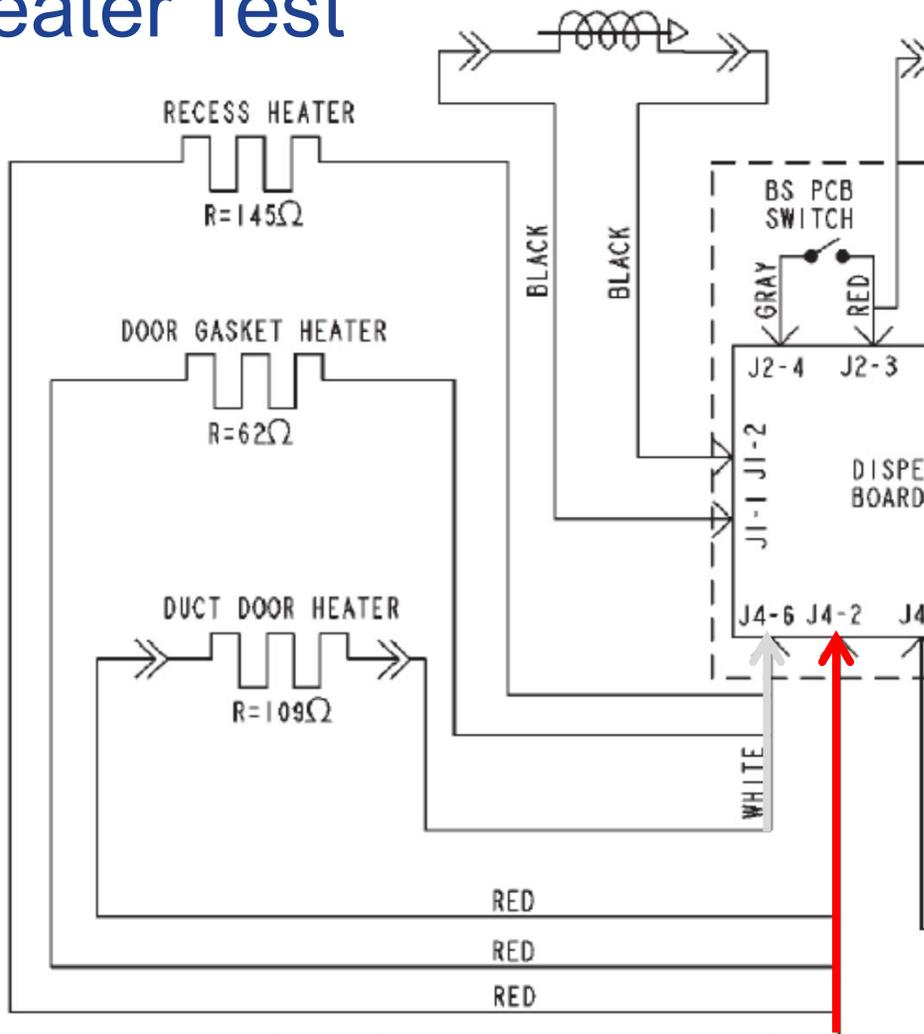
Heaters operate based on temperature settings i.e. FRZ setting of 5 or higher = 100% "On" time except during ice dispense. (Circuit can be tested at dispenser board also. Wh/Red)
