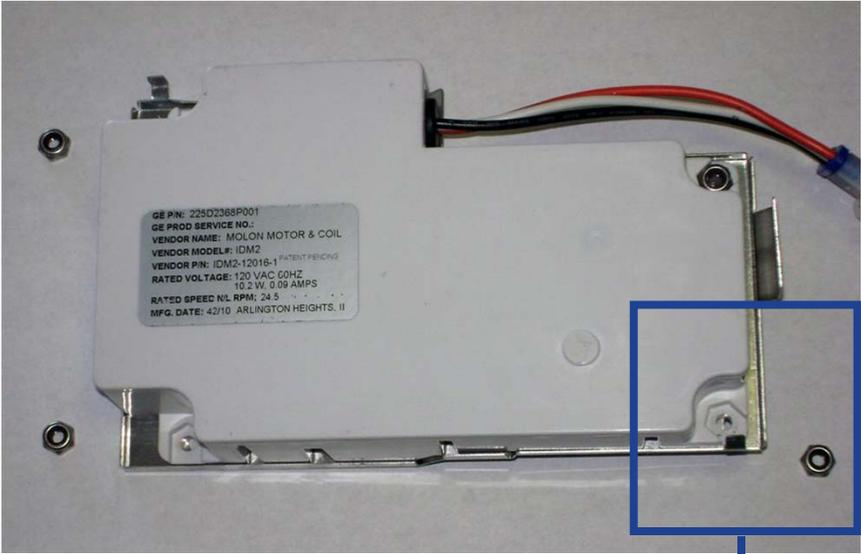
Remove auger fork by removing nut
