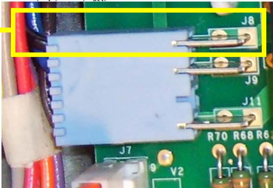
Air Duct and Supply Duct heaters use J8 (compressor) relay
