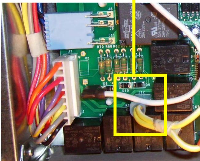
Off during ice dispense to reduce power supply output and remain off for 5 more seconds after ice dispense completed.
