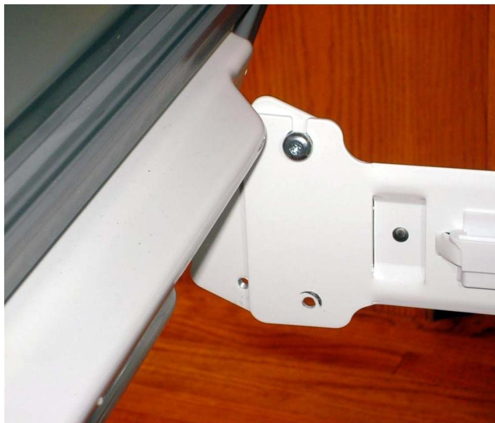
**Remove outer panel by removing the lower T30 torx screw. Loosen the top one and lift panel up and off.**
