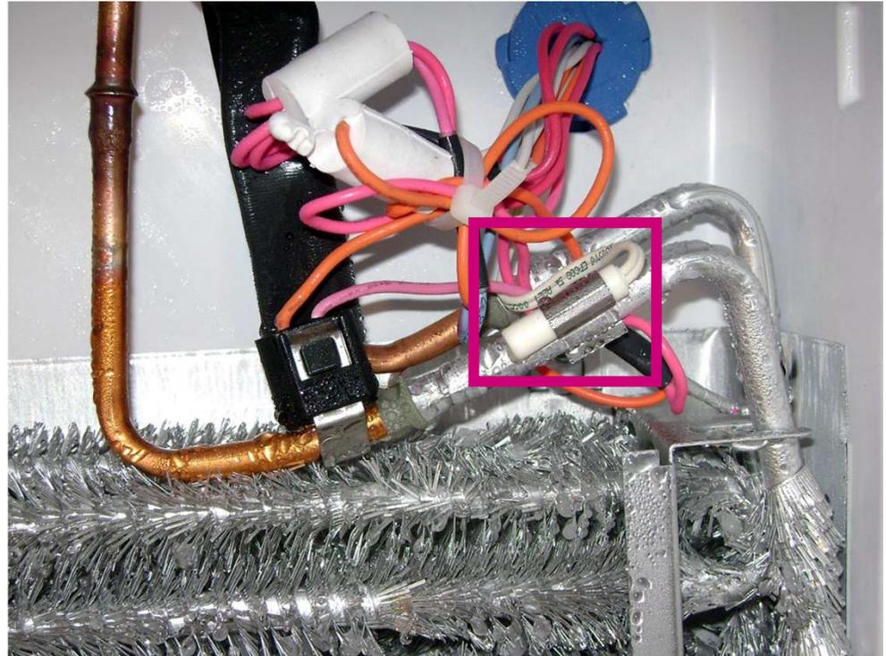
Evaporator thermistor clipped to tubing.
