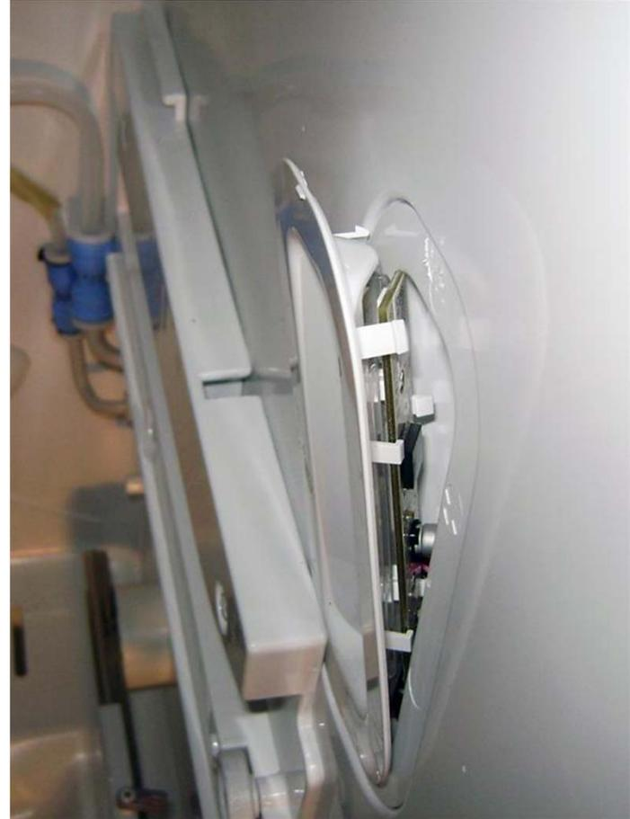
Gently pry with putty knife or small flat bladed screwdriver at the top “**notched**” end. Assembly snaps out and lifts slightly up from the bottom.
