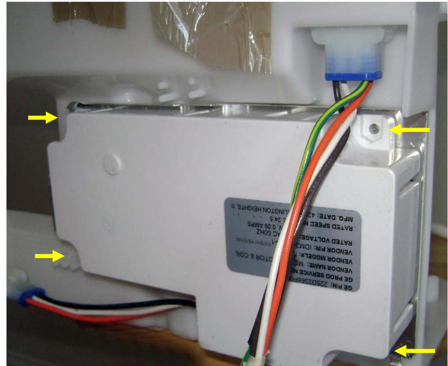
Remove 4 mounting screws and nuts located in the 4 corners.
