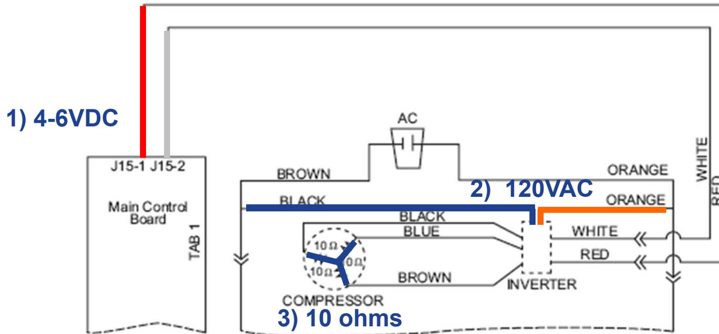
**Note:** When measuring signal voltage (from the main control board) at the inverter, a reading of 4-6 VDC will be measured with all wires connected. If the inverter wiring is disconnected, the board output will measure between 10-12 VDC.
