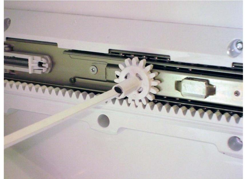
To remove side wall tracks, start by removing the roller guide bar. Remove small black locating pin and slide bar to right and remove from rollers.
