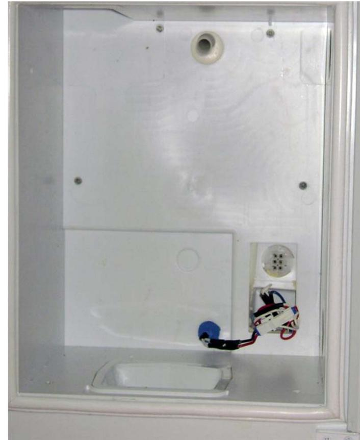
**Auger motor removed**
