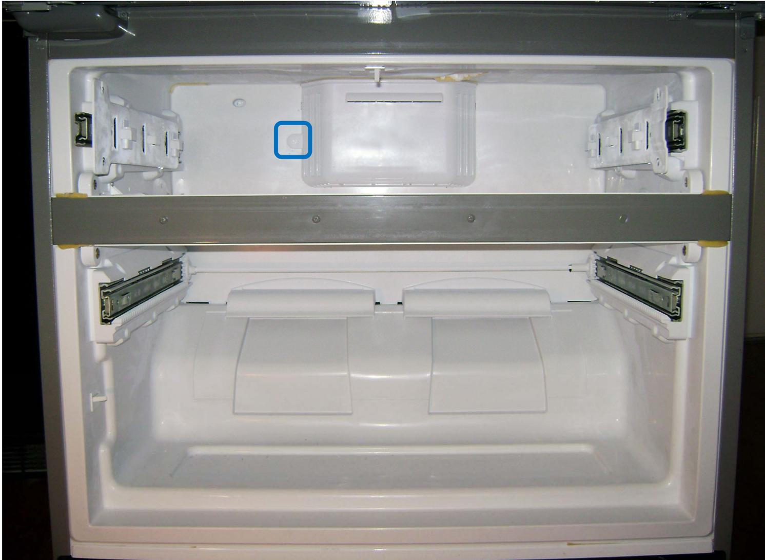
Remove fan cover screw and swing off
