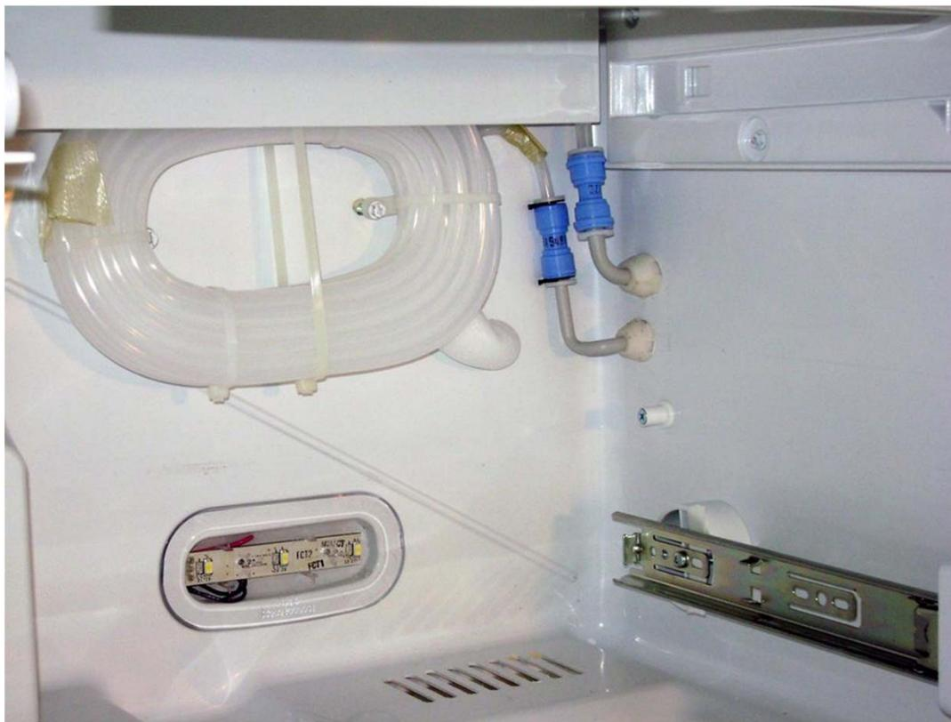
Water line connections on lower right hand corner of FF section
