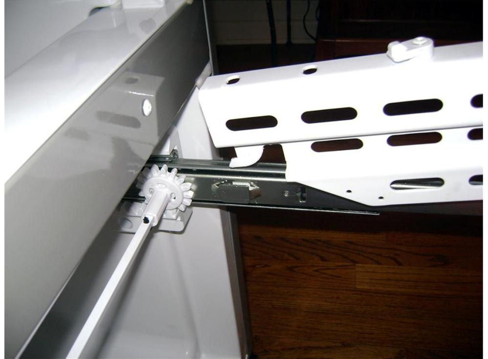
**With both screws removed, lift up on drawer front and disengage from rear slots.**
