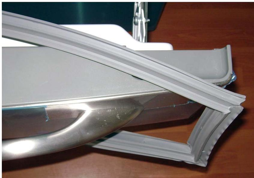
**Gasket can be easily removed by peeling away from inner panel and sliding over the outer panel.**
