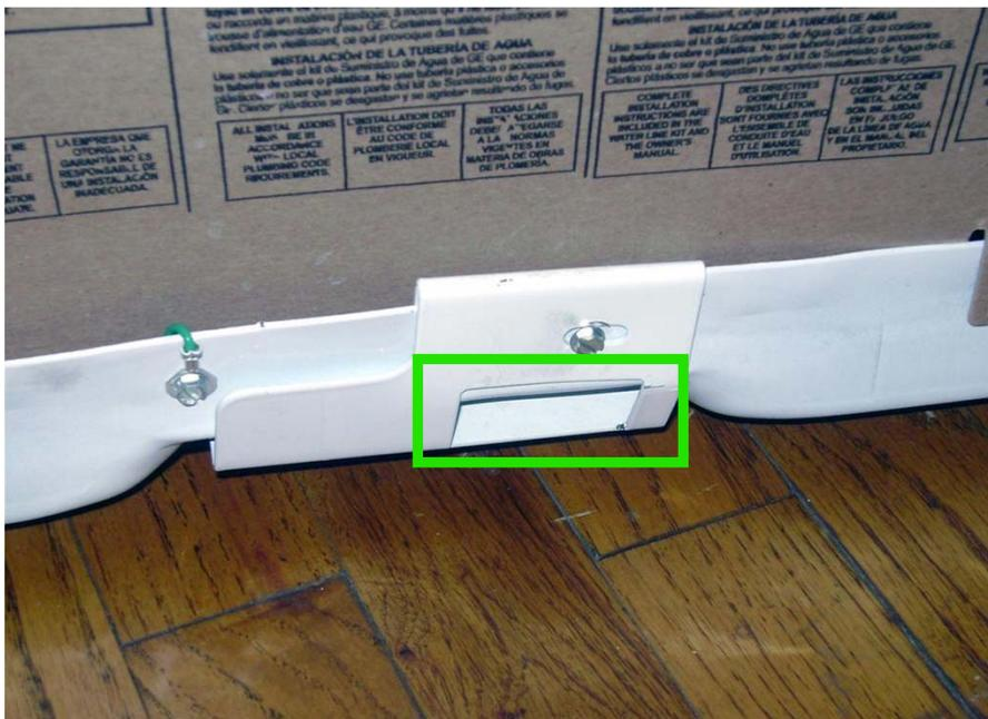
Anti-tip bracket fits into opening when refrigerator is slid back into place.
