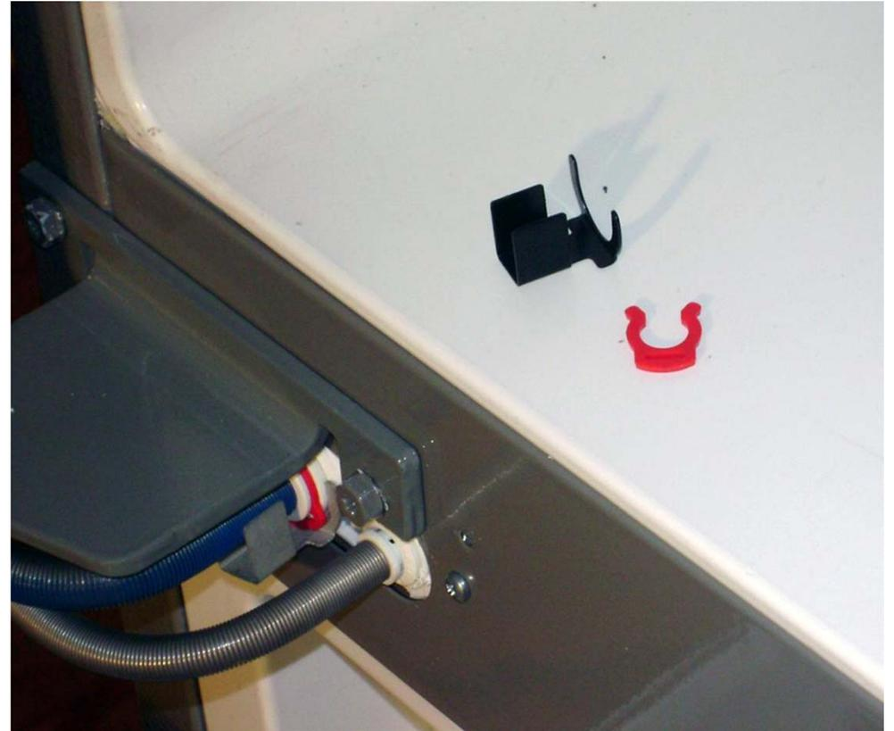
**Remove black shield and red clip for each water line**
