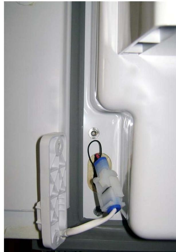
Check heater for 24  $\Omega$  resistance or 13 VDC
