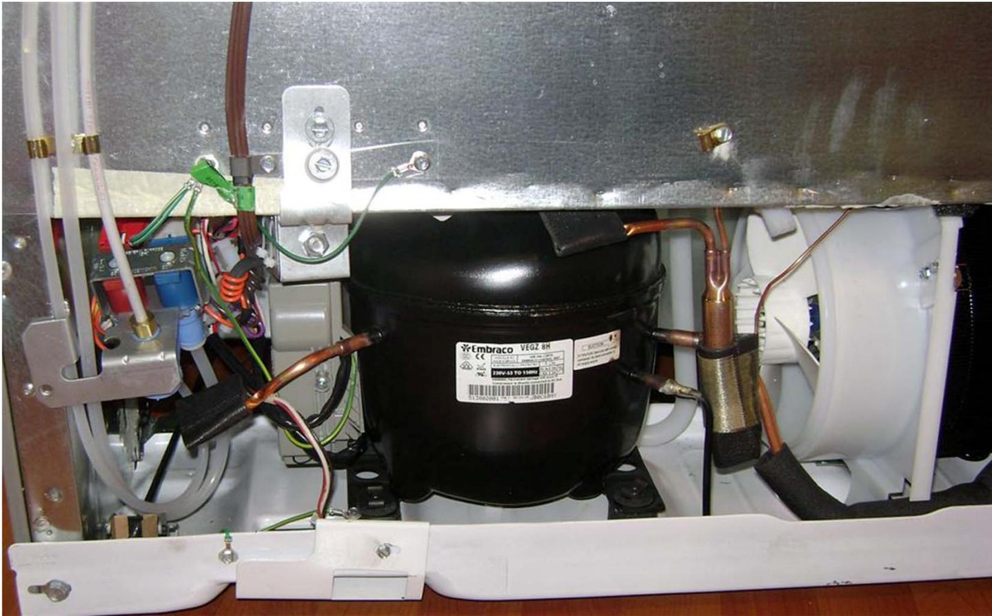
Three speed / three phase inverter controlled compressor
