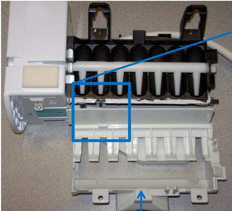
**Note fill cup assembly removed and upside down for better viewing.**
