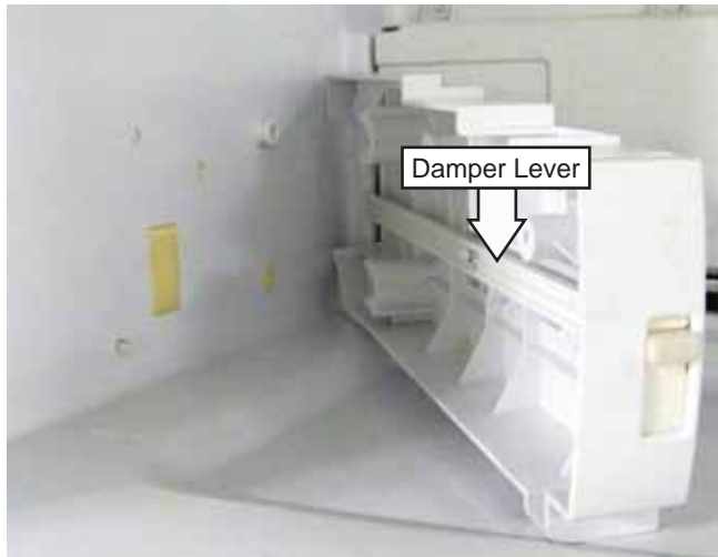
Damper lever shown in closed position
