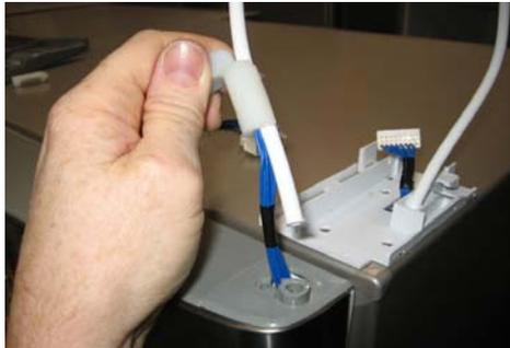
Fit harness to bullet supplied with replacement door and tape harness to bullet
