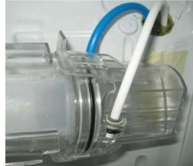
Hoses are accessible once tank is removed.
