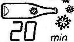
Bottle Chill allows the customer to put a bottle in the freezer for a designated amount of time. When that amount of time has elapsed an alarm will sound telling the customer to take the bottle out of the FC. The Freezer automatically changes to it's lowest set point.
