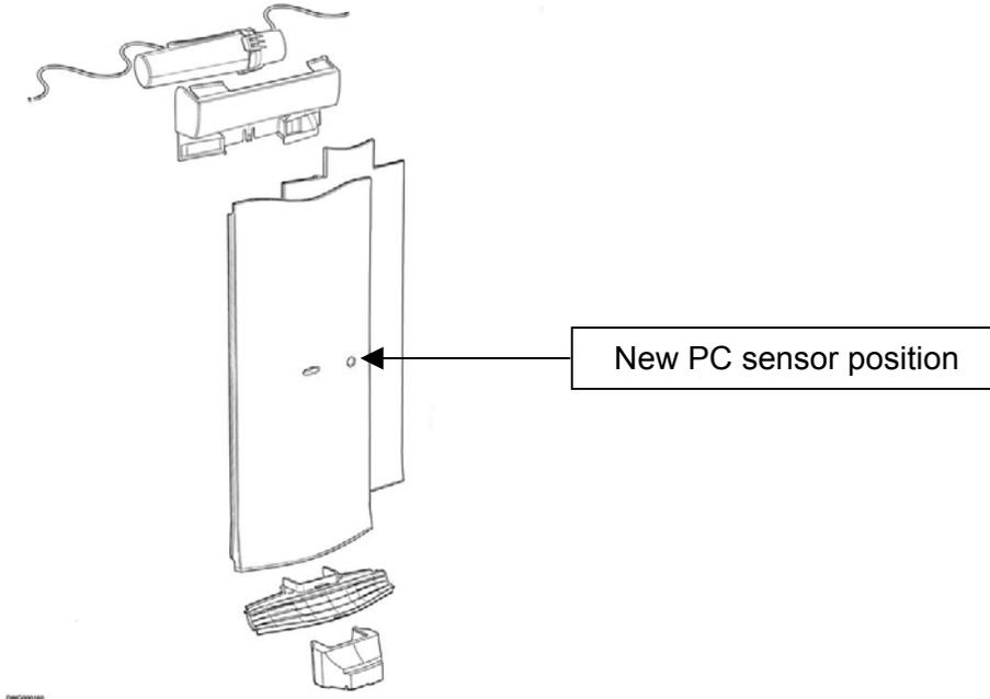
Note: When replacing door ensure the collets are refitted and the product is water tested after completion of repair.
