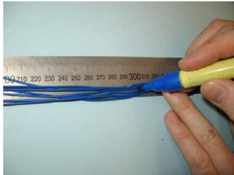
The mark on the harness is to be placed in the middle of the guide.
