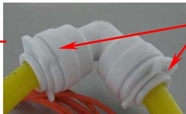
Collet Locking clips in position – remove left hand clip to remove door.
