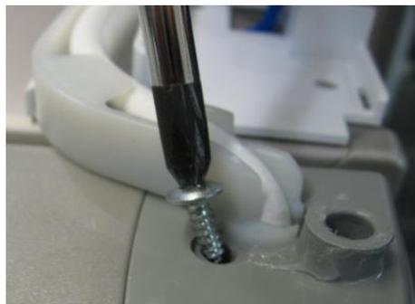
Turn guide 90° to door to remove guide from housing
