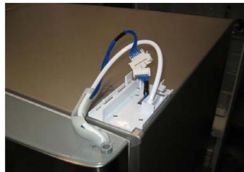
Refit guide to hinge – ensure tab lines up with cut out
