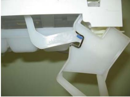
Bin lever in down position - when in this position icemaker will not rotate/harvest.
