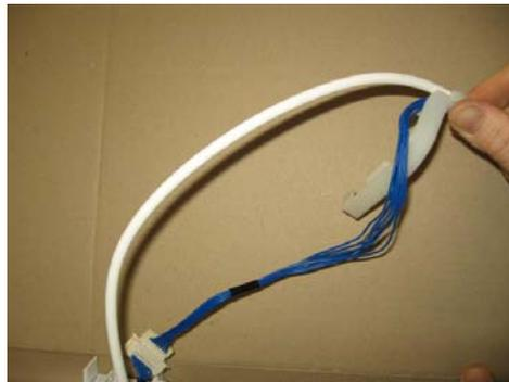
Using the bullet, place the RAST connector and hose as shown.
