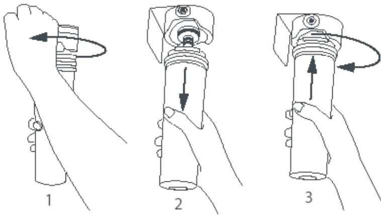
Fig.11 Changing the water filter cartridge
