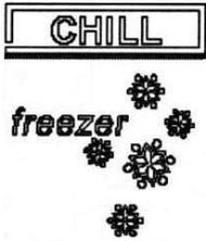
Freezer chill is a function that rapidly freezes food in the FC by temporarily dropping the freezer to its coldest temperature set point for a 12-hour period.
