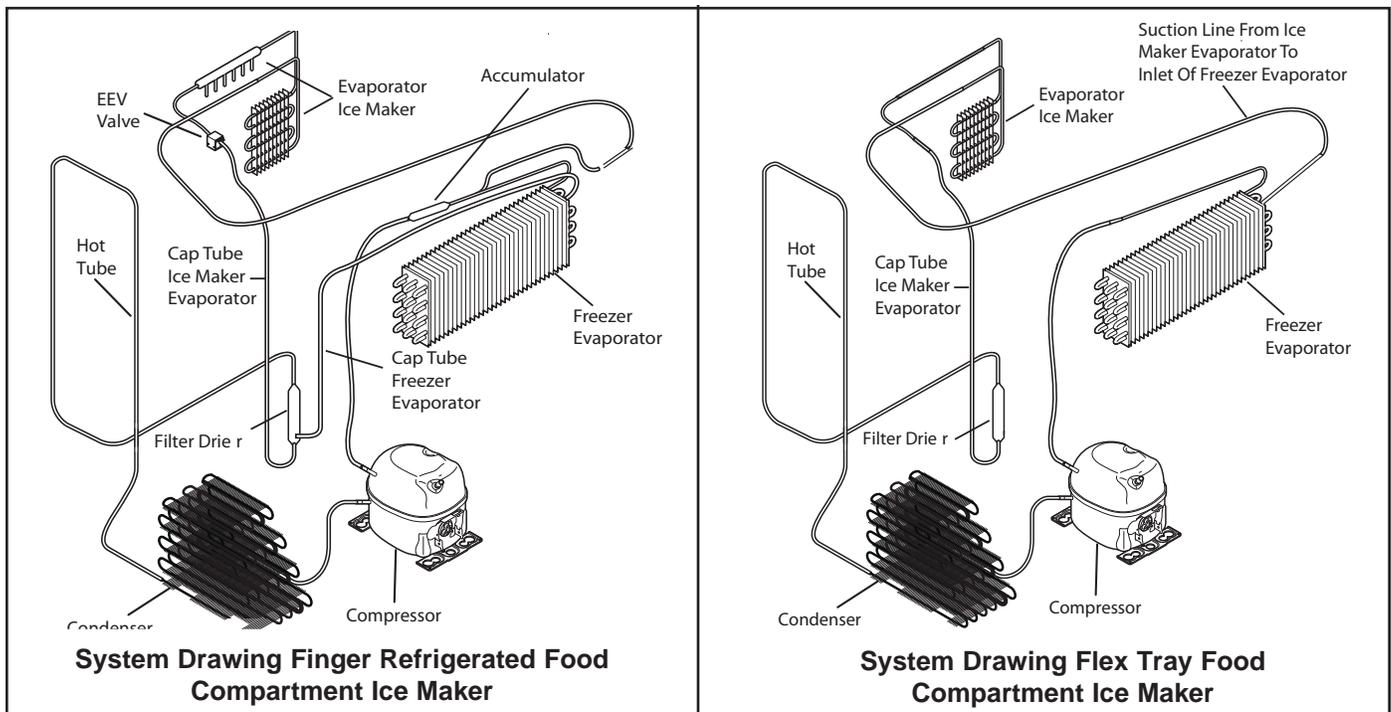
Figure 7-3 . Automatic Defrost Models
