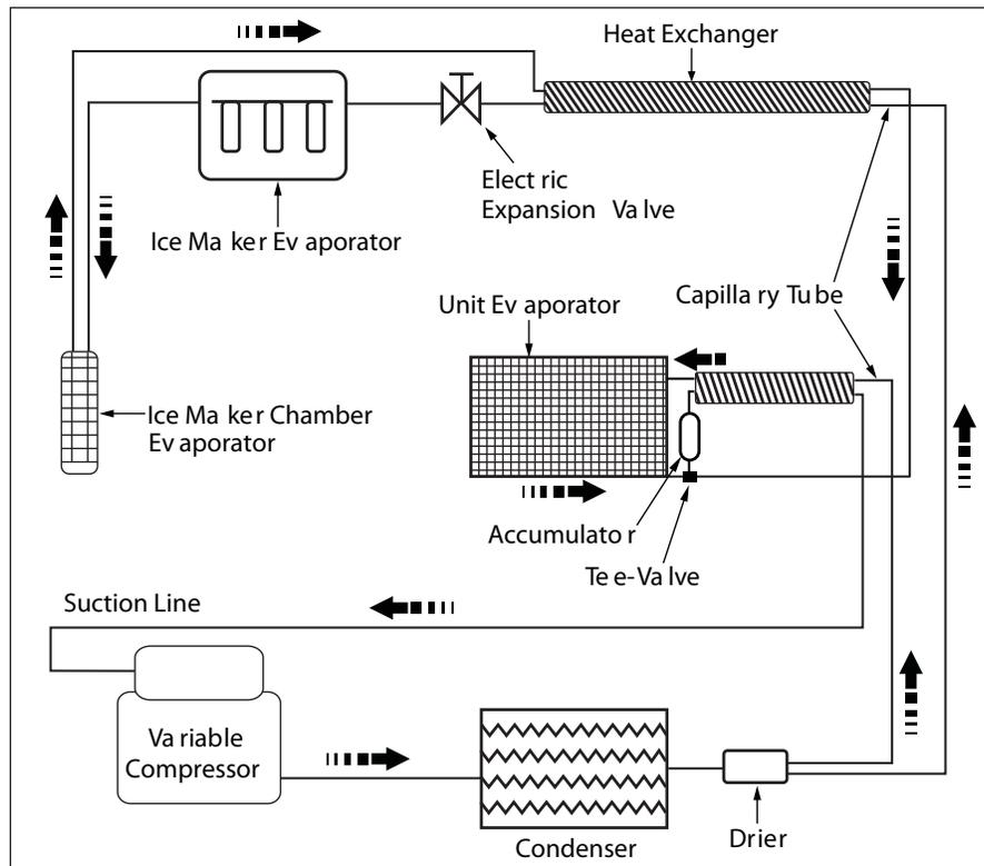
Figure 4-11. Ice Maker Refrigeration Flow Schematic
