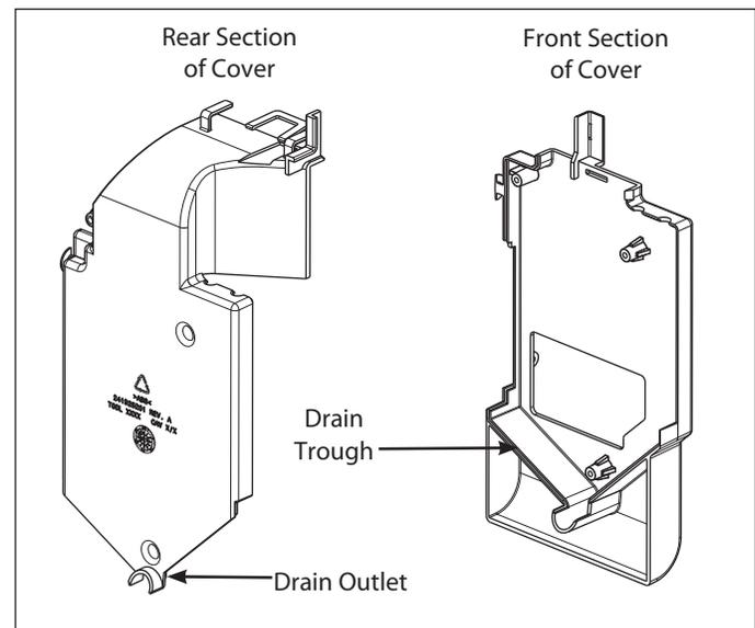
Figure 4-10. Icemaker Water Drain
