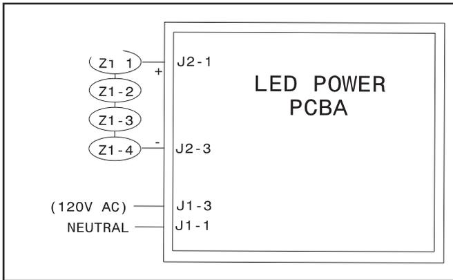
Figure 3-15. LED Power Board For Lighting In Food Compartment
