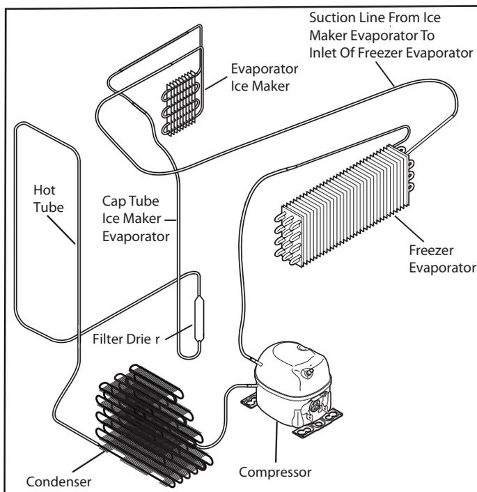
Figure 4-2. Ice Maker Refrigeration Schematic
