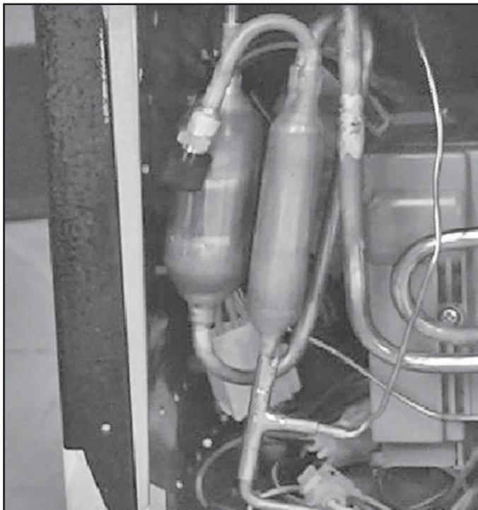
Figure 7-16. Two Stage Drier Kit
