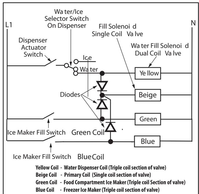
Figure 5-2. Diode Schematic
