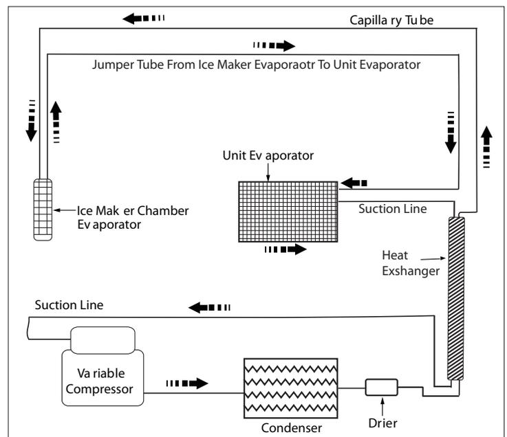
Figure 4-7. Ice Maker Refrigeration Flow Schematic
