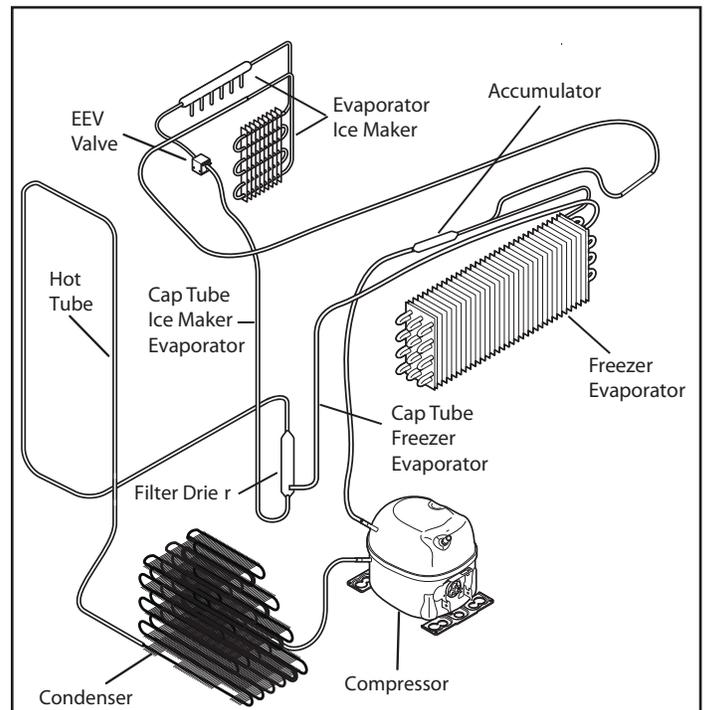
Figure 4-9. Ice Maker Refrigeration Schematic
