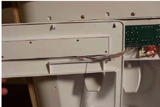
Unplug the wire harness from touch panel to board.
