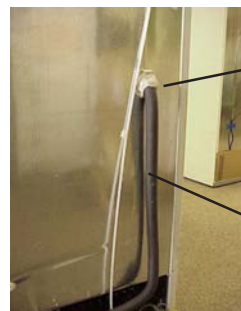
Push the heat exchanger through the hole in the cabinet.
