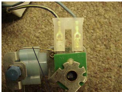
Terminal on Coil is Installed Over Top of Terminal on Left Side of Plug
