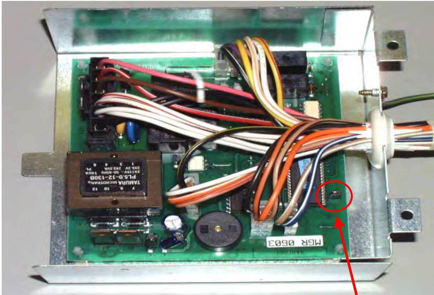
If jumper is left on board it will cause the display to go into the test mode when unit is powered up. Lasts approx. 20 seconds on power-up. Refrigerator then operates normally
