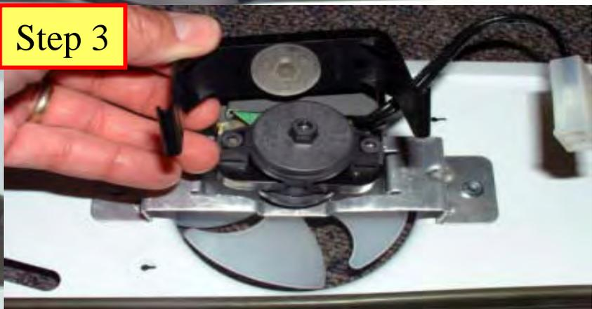
Remove bracket and pull fan blade
