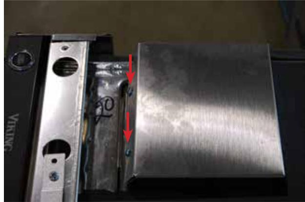
At this time the vent assembly can be removed from unit by lifting up and out, from the top of unit.
