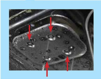
Remove the panel and set aside to gain access to the mounting screws for the vent assembly, remove screws as shown in photo below.
