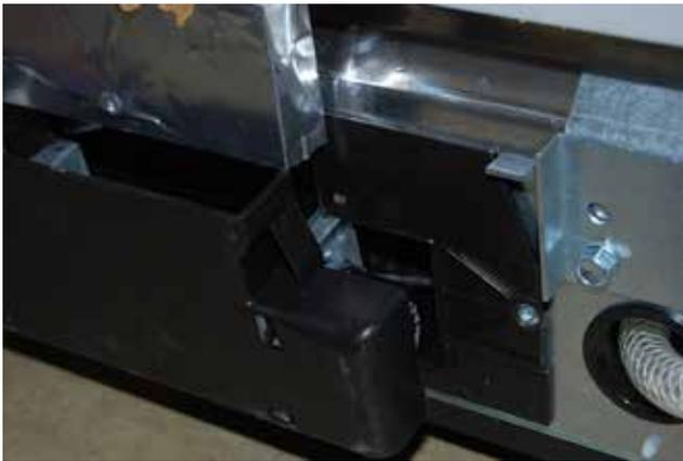
Pull blower assembly out towards you slowly as shown above. Disconnect blower motor connection as shown below.
