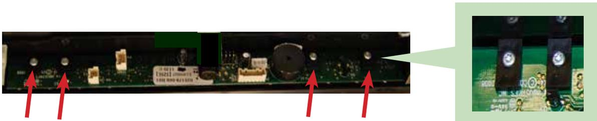
Remove the four T10 Torx screws as indicated by arrows in photo above, remove user interface board from control panel assembly.
