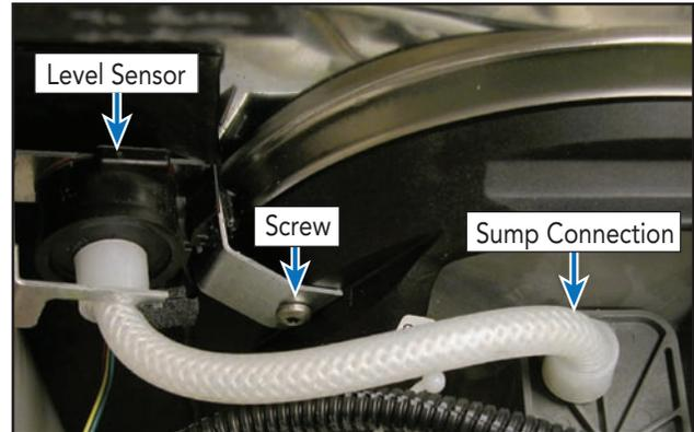
The image below shows the three wire connector to the level sensor.
