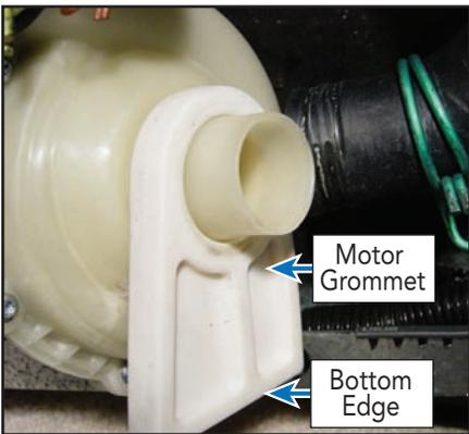
**Note:** that there is a white motor grommet over the pump opening. Make sure it is back in place and bottom edge is facing base pan before reassembly. (The second right image on page 40 shows proper position of grommet).
