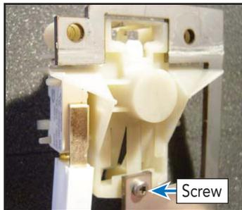
Inner Door Duct Assembly—450 model
