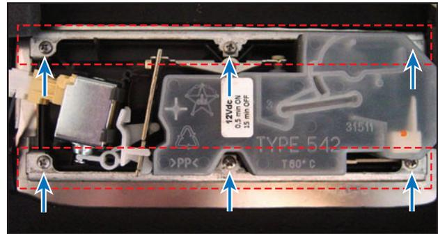
The image below shows the solenoid unplugged to remove the dispenser assembly. Unplug the two-wire connector plug in order to remove the dispenser.
