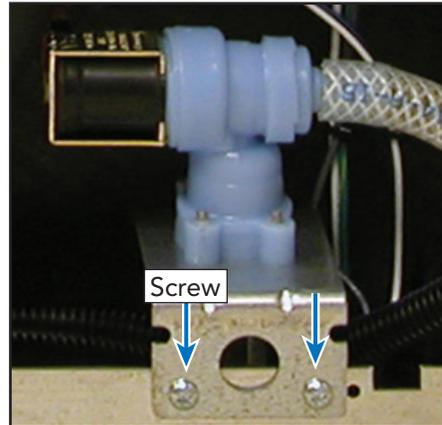
Remove the two screws shown above and remove the fill valve from the base.
