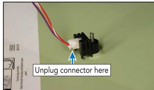
**Note:** Place base pan in a secured area. Take care not to damage the sensor.
