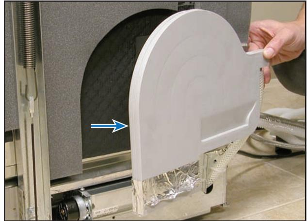
Remove the two remaining TORX® screws that are indicated below. Now remove the heater assembly.
