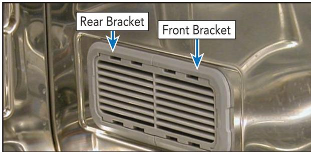
Using a flat blade screwdriver, gently pry the locking brackets off the inlet assembly. Both the front and rear brackets are the same. The rear bracket must slide backwards to remove and the front bracket slid forward to remove.
