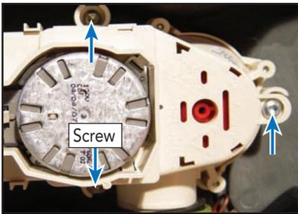
Remove the diverter from the sump assembly. The image below (left) shows the rear of the diverter and below (right) shows the sump area with the diverter removed.
