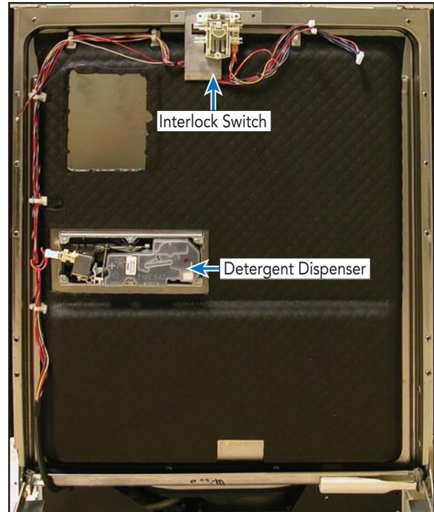
From here you can test the door interlock switch and the detergent dispenser.
