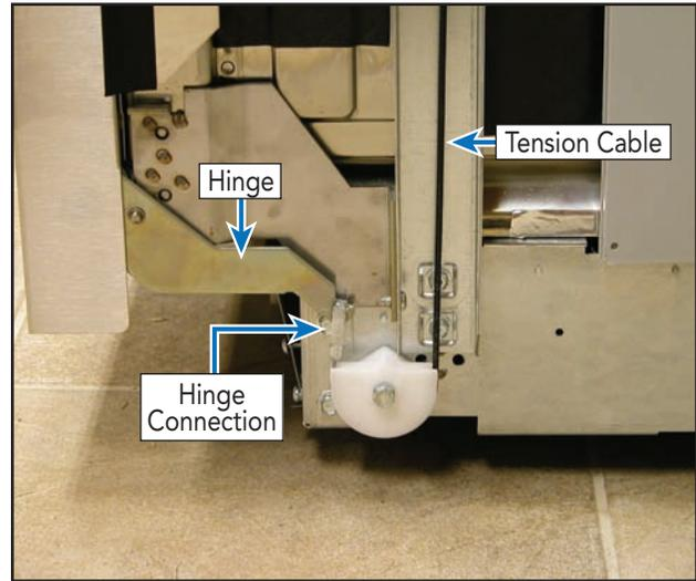
Remove two screws which connect the inner door at the hinges.
