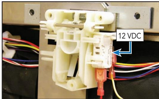
If replacing the switch, remove the bracket from the old switch and reinstall on the replacement latch assembly. Remove the TORX® screw shown below.
