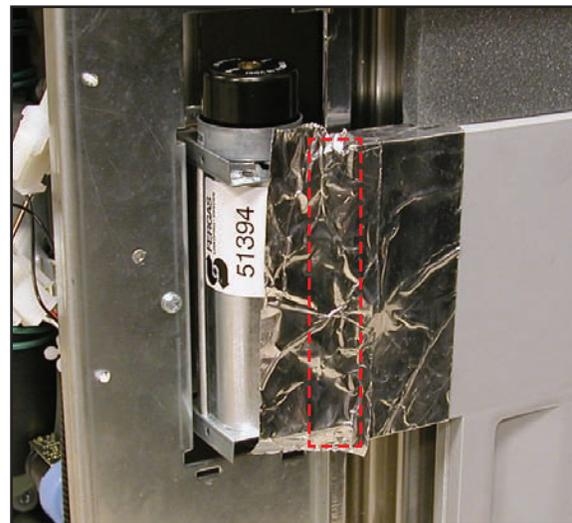
There are four screws in total that need to be removed in order to remove the heater. The following images will their locations.
