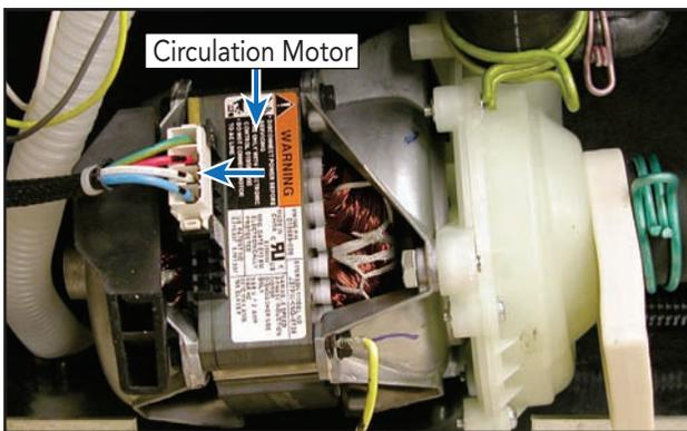
P5-1 and P5-2 sends 120 Volts to the motor controller. The motor controller then converts the voltage to operate the three-phase motor.
