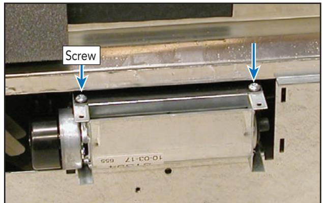
**Note:** In the image above, the air/water Inlet assembly is detached from the machine.
