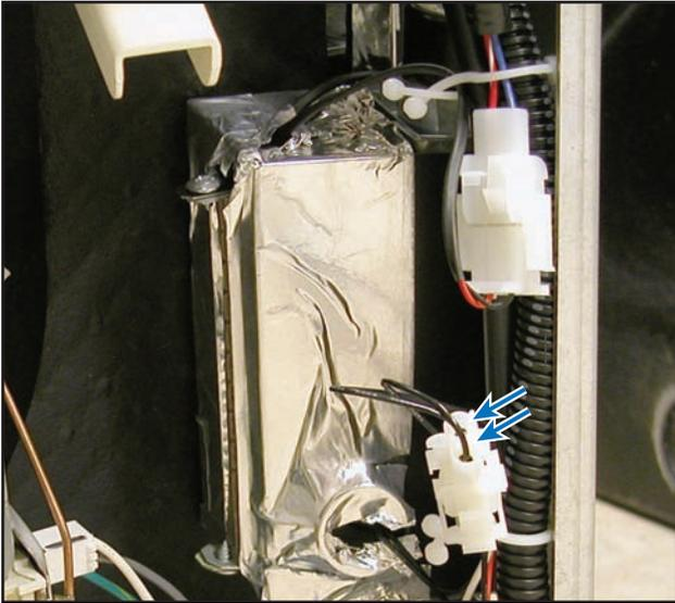
Remove the heater housing to expose the blower motor.
