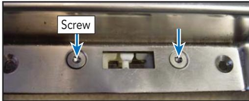
Remove the latch mechanism and unplug the 2-wire connector plug from the micro switch shown below.
