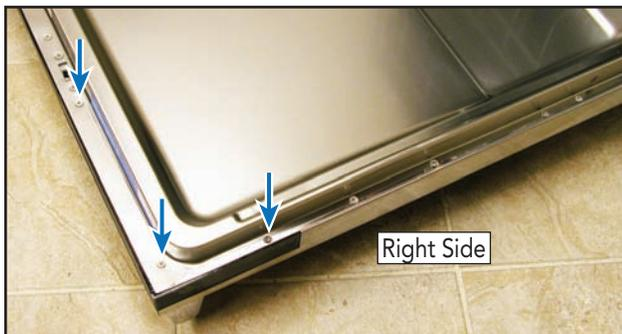
**Note:** With the outer door panel and the control panel removed, access to the user interface is gained.
