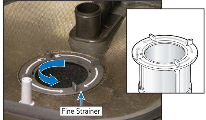
Lift fine strainer out and repair or replace as necessary. Reverse the procedure to reinstall the fine strainer. Make sure the fine strainer locks (using pressure, press down and turn).
