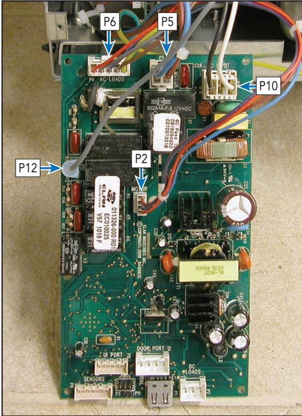
**Note:** It is recommended that the control be taken out before removing the motor control board. It makes it easier to handle removal.
