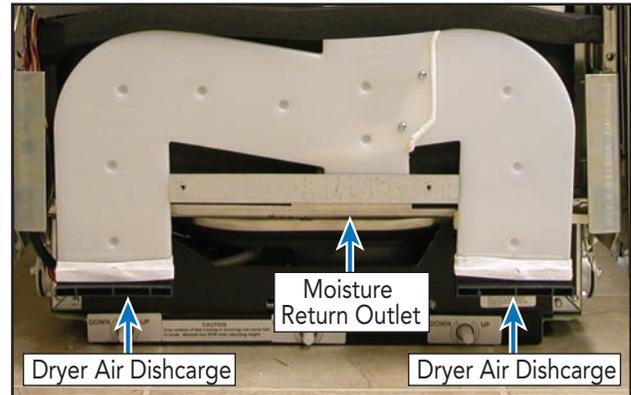
The moisture return outlet of drying vent assembly is held in a retaining bracket which is secured to the inner door liner. First remove the four screws from the active vent. Unscrew active vent from the inner door and remove the vent assembly.
