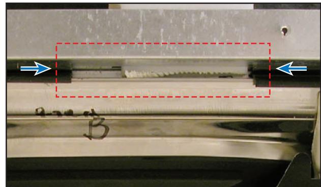
The two arrows above show the vent in position. The rectangular red lines shows the area where the condensed moisture returns to the sump area.
