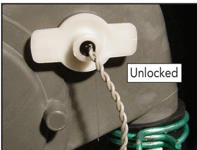
While grasping the tabs, pull the sensor out of the sump assembly as shown.
