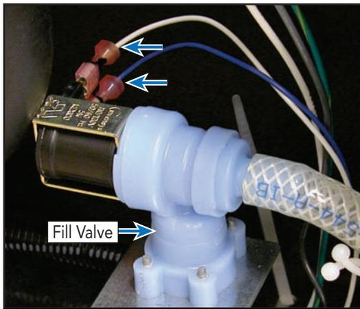
**Note:** Resistance reading is taken at valve (shown above) not control board.
