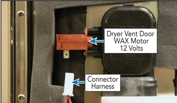
**Note:** The vent door is normally open when the dishwasher is not in use. When switched on, the WAX motor will heat up and close the internal door during a wash cycle and open during the dry cycle.
