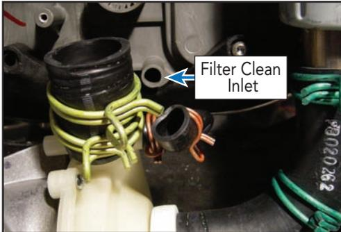
The image below shows the hose disconnected from the pump.
