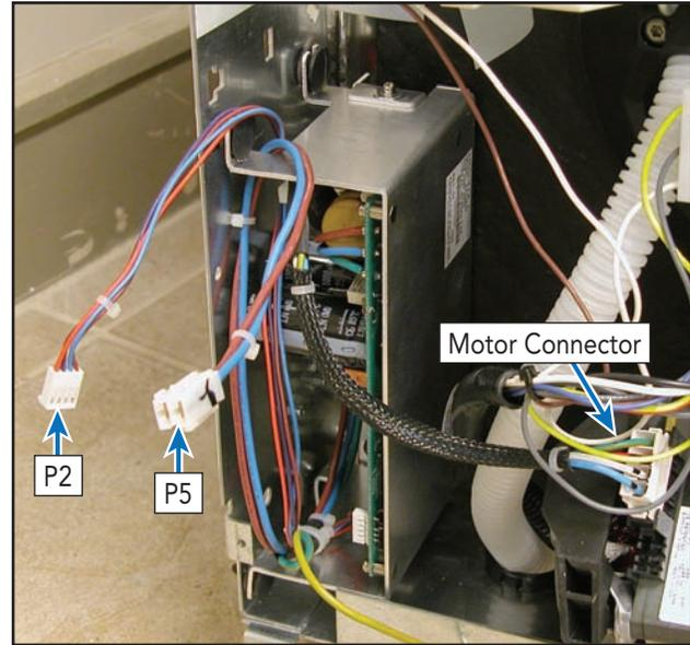
P5 provides 120-volt AC power to the motor controller. P2 provides the control signal voltage between the control board and the motor controller.
