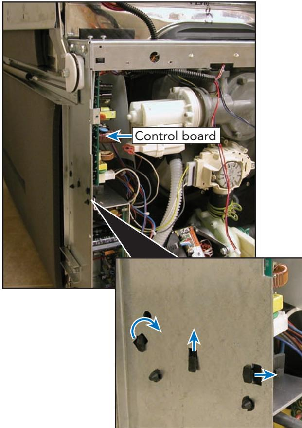
Now carefully pull the board down and release from the front.
