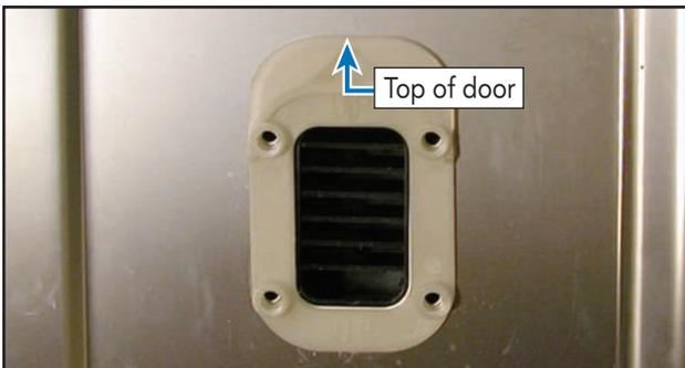
The image below shows the vent spacer removed.
