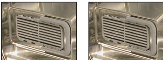
With the locking brackets removed, pull the fill chamber away from the right side of the unit.
