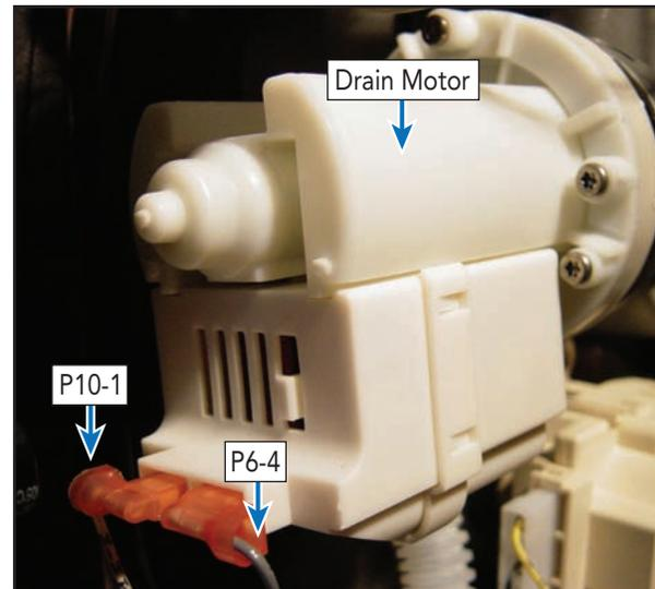
**Note:** Resistance reading is taken at pump (shown above) not control board.
