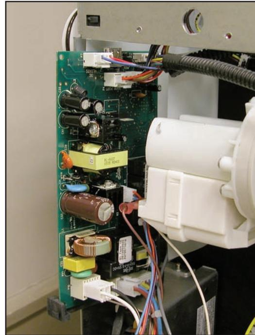
Disconnect the P7, P4, P8 and the P9 connectors from the board.
