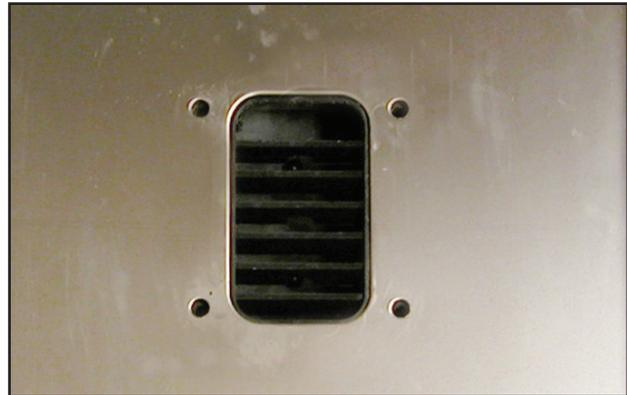
Now close the door and you can now remove the dryer door vent mechanism as shown below. Be sure that when reassembling the vent that the lip edge of the vent is positioned properly in the opening of the door liner. Failure to do so could cause a water leak inside the door.
