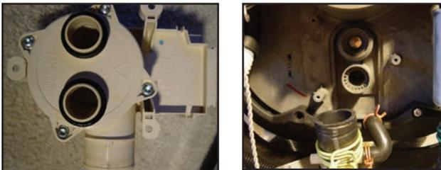
**Note:** There are two O-rings that must be put back. Failure to do so will result in a water leak.
