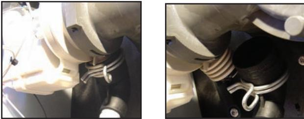
Next, release the drain motor from the sump assembly. Locate the release tab (indicated by the yellow dotted line, below left). Using a flat blade screwdriver, bend the tab in the direction shown by the arrow (below right) to release the pump from the main housing. Grasp the pump and rotate clockwise and the pump can be removed.
