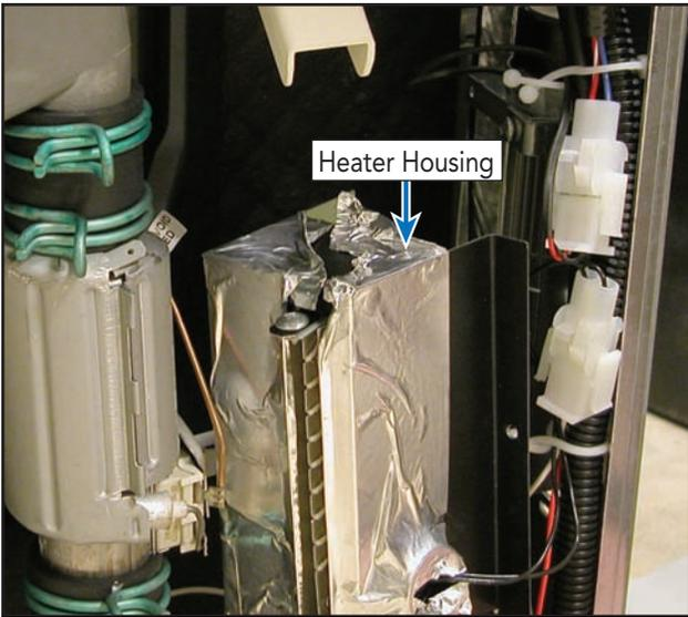
**Note:** When reassembling the heater housing, you must replace the aluminum tape that was removed during disassembly. Failure to do so may cause improper air flow across the heater.
