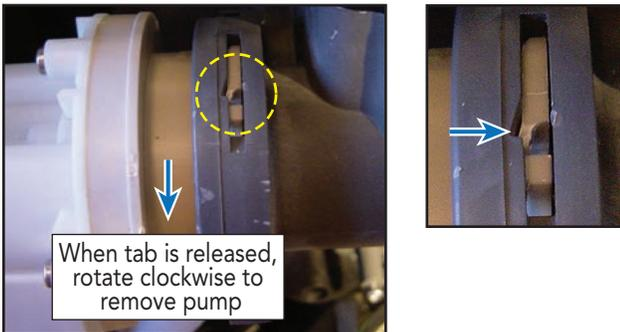
When reinstalling pump, make sure to bend the tab back in place to lock the pump into the sump housing.
