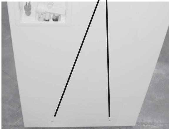
7. Carefully spread the front cabinet sides for clearance around the tub flange.
