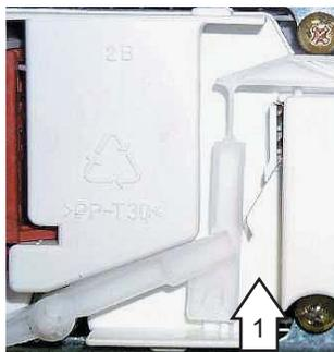
When deactivated (2), the lever returns down the left-hand path and comes to rest under the notch in the center of the connecting rod.
