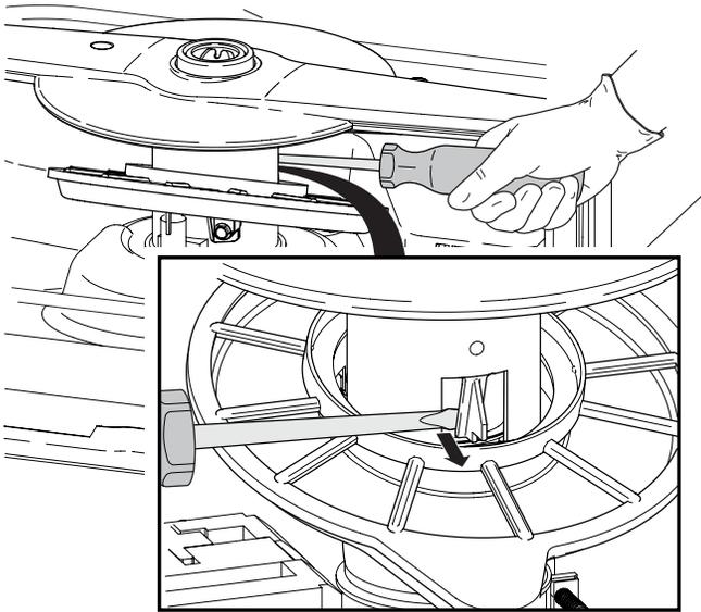
3. Remove the 1/4-in. hex-head screw that connects the spray arm base to the fine filter assembly.
