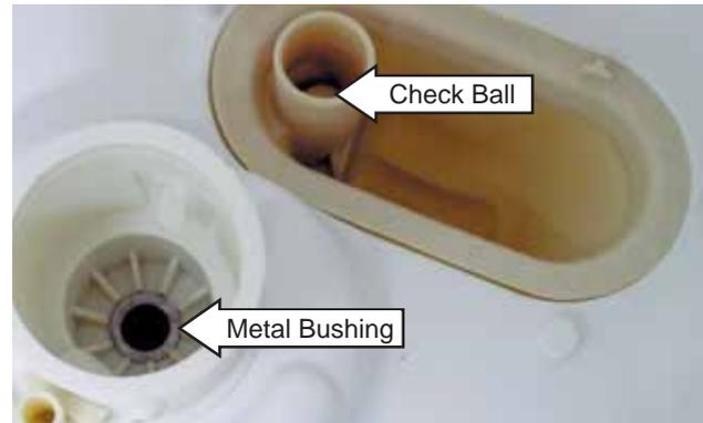
2. Lift up on the edges of the sump boot, squeeze inward, and push the sump through the opening in the tub floor.
