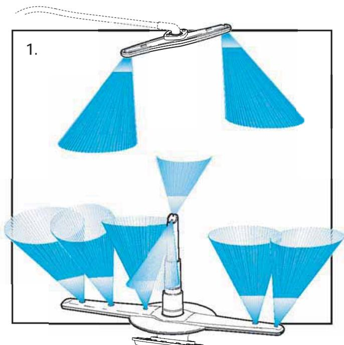
1. **5-Level Wash** - Models containing an upper spray arm have 5 wash levels. These models include the PowerTower™ spray and the new lower spray arm.
