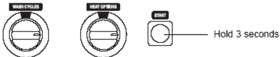
To access the output latching mode on Rotary Models 6600, 6605 align the wash cycles and heat options indicators on the knobs with the Start/Cancel button (both knobs horizontal and pointing towards start/cancel button, then press and hold for 3 seconds the Start/Cancel button when no program LEDs are on. Both LEDs are to turn on for 1 second to indicate that the output test mode has been accessed.
