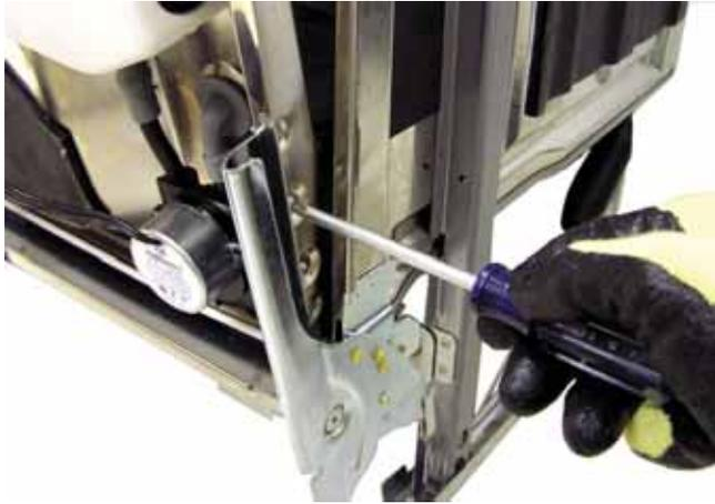
3. Remove the grommet from the inner door panel and unplug the tube from the reservoir outlet.
