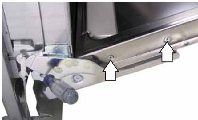
7. Slide the inner door panel off the door hinges.
