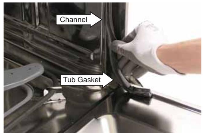
**Caution:** When installing the tub gasket, run your finger over the gasket, assuring it is smooth and even for a proper seal.
