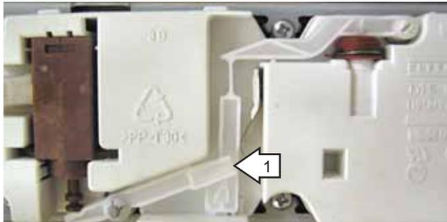
When the module is deactivated, the lever returns down the left-hand path and comes to rest under the notch (2) in the center of the connecting rod.
