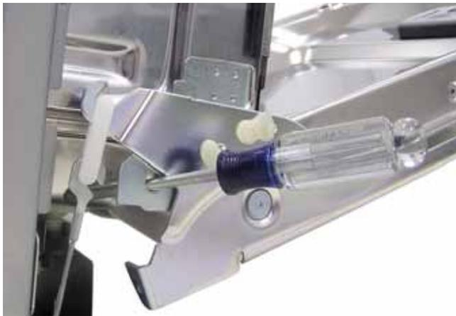
6. Remove the 4 Phillips-head screws holding the inner door panel to the door hinges (2 on each side).
