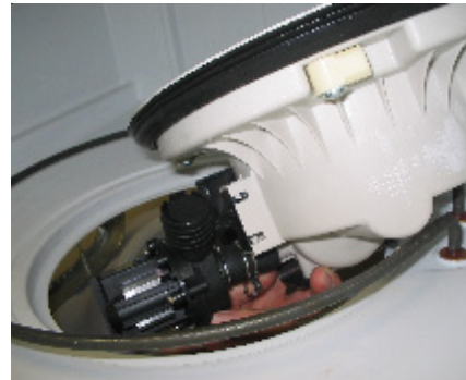
Lift sump to the 2:00 position to remove
