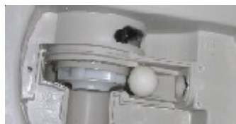
Check ball moved up ramp.
