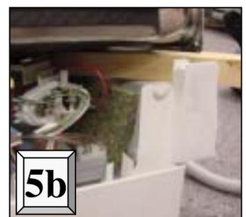
**CAUTION:** Its not recommended to turn dishwashers upside-down for tank access. When dishwashers are turned upside-down, water can flow into the diaphragm of the water fill assembly and cause water to not fill properly.
