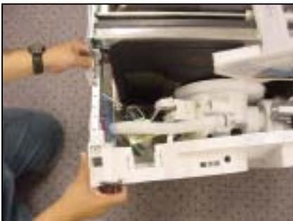
***Carefully pull base away from tank & sump***
