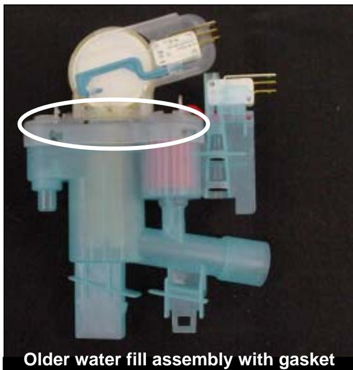
**NOTE:** Older water fill assemblies required a gasket between the upper and lower housings. Newer ones do not require gaskets and are a drop-in replacement for older ones.
