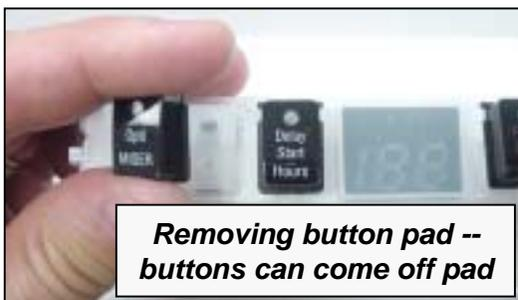
*Removing button pad -- buttons can come off pad*
