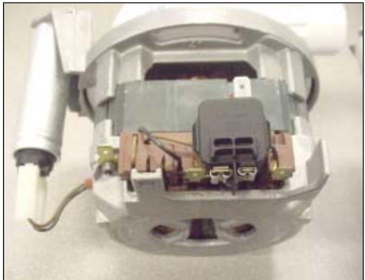
**TECH NOTES:** New motor starter # 423023 (15Ω) has a larger resistance to limit current draw through pump motor start windings. Winding temperatures are reduced, but starting torque is reduced as well. So, new motor starters (# 423023) should never be used with new circulation pumps (# 437345).
