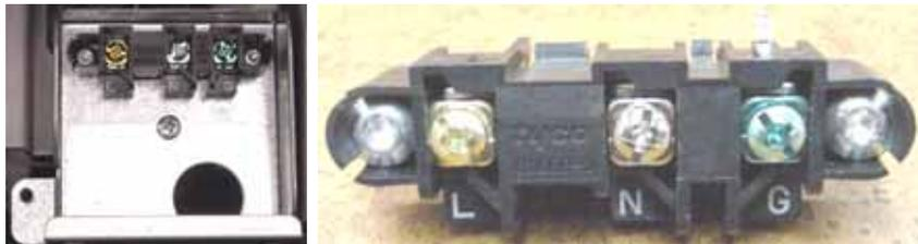
Terminal blocks can't be installed in the field – the terminal box assy with terminal block must be ordered. The terminal box assy assures the terminal block is properly grounded to the terminal box.
