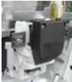
Other than occasional misalignment, the only door latch repairs will be replacing microswitches. Door latches are held in place in console (frames) by tabs. It's important latches are properly seated in consoles and tabs are fully inserted into latches.
