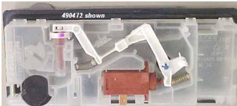
During each wash program, the wax motor opens twice, once to dispense detergent and again to dispense rinse-aid. The wax motor opens the same -- linkages open the detergent door & operate the rinse-aid dosage plunger. Dispensers can have reed switches or optical rinse-aid sensors.
