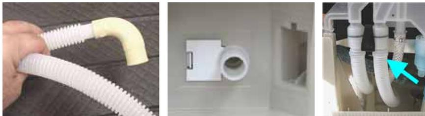
To remove the internal drain hose, remove a white plastic hose lock and pull the hose from the water level control.
