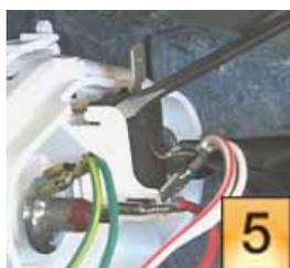
**TIP:** If needed, use rinse-aid to lubricate gaskets to make it easier to assemble heater to sump and pump.
