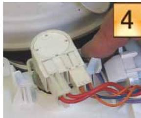
5. To remove flow switch, carefully pry housing away from switch (until tabs clear switch), then snap switch out. Note flow switch can be removed from right side without flipping dishwasher upside-down.
