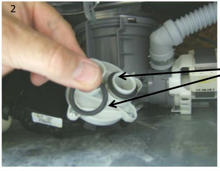
Before installing the new diverter be sure to install the “O” rings from the old one onto the new one (see illustration) or the new unit will leak.
