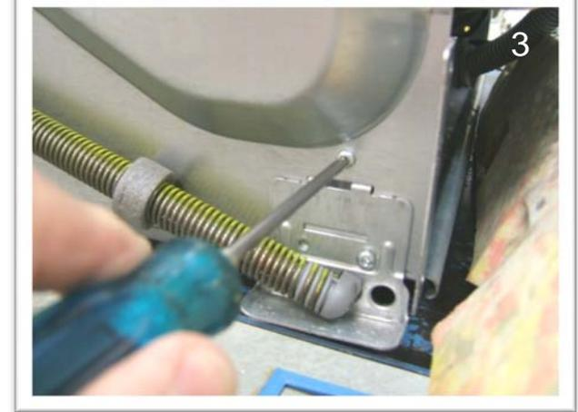
With a straight blade screwdriver rotate cover counter clockwise to remove. Remove single screw on outside and two from the inside of the tank.
