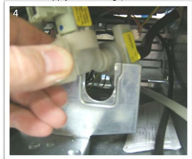
Slide the valve out of the bracket
