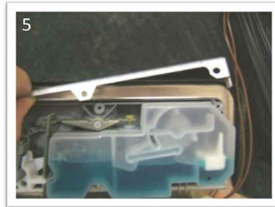
Remove the remaining screws holding the upper and lower clamps.
