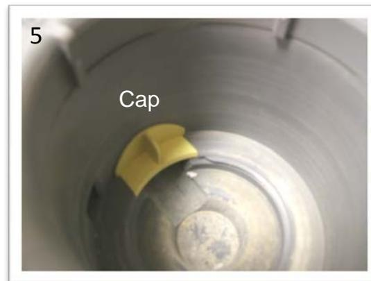
5 Sump drain cap sits down in the sump area inside the outlet to the drain pump
