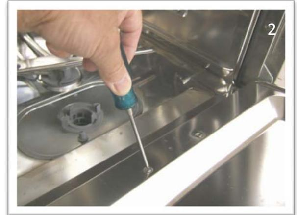
Remove the 2 bottom screws first
