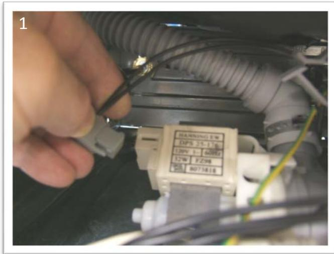
To remove the drain pump first disconnect the Molex connector.
