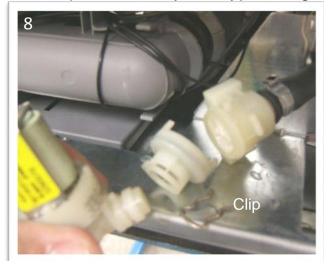
The flow meter is connected to the rear of the fill valve. The whole assembly can be replaced by removing the hose which goes up to the air break. A new hose clamp will then be needed to reconnect the new assembly. Or the flow meter can be disconnected from the fill valve via the retaining clip or with the bayonet fitting
