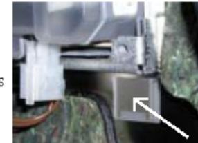
3. Refit the thermistor. Make sure the thermistor rests against the spacer.
