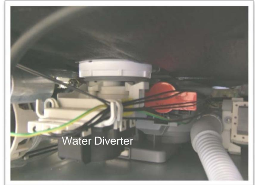
Circulation motor/pump is removed in the same manor as the 3,000 series, however there is less room to maneuver due to the taller tank. It may be easier to remove and replace the motor/pump as a complete assembly.
