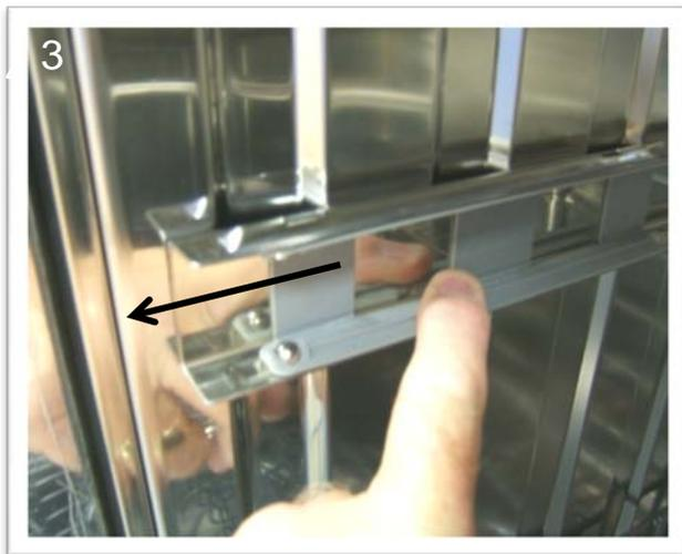
Slide out the ball bearing plastic holder which should contain 4 bearings. Check the bottom of the tank for broken off plastic pieces or ball bearings which may have fallen out.
