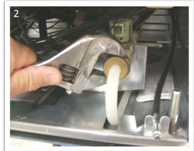
Unscrew supply hose fitting (turn off water first)
