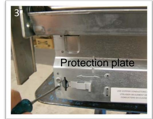
Remove eight screws, four each side (2 are underneath), to release the protection plate
