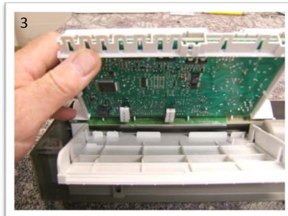
After removing the wire connections and removing control panel from the unit, lay it down on a protected flat surface. Not all control boards can be removed from the panel intact, for example the FI unit shown above. In this case separate the casing by using a flat blade screwdriver and prying the tabs apart see (2)
