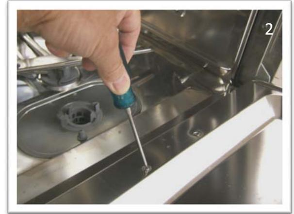
Remove the 2 bottom screws first
