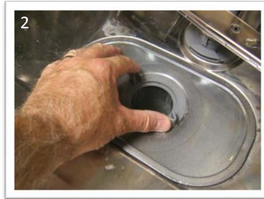
2 Rotate fine mesh filter counter clockwise .
