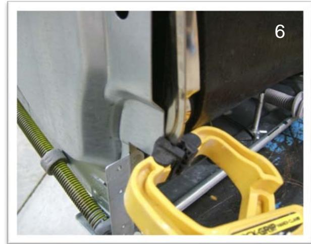
Block side wall away from tank, and slide the air break out from its location. When reinstalling make sure the seal is in place and use a clamp to pull side support to tank so that screws will engage.
