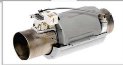
Access to the heating element is achieved from the rear of the unit in the same manor as the circulation motor/pump. The heating element is suspended between the circulation pump housing and the sump housing and is secured with rubber seal inserts. It is a push fit and there are no clamps. The circulation motor will have to be removed first in order to pull the heating element off of the sump.
