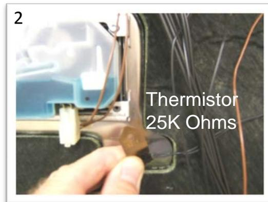
Remove thermistor from right side of lower clamp (3,000 series only)
