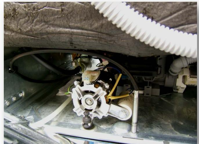
The circulation Motor has a resistance of **22 ohms** and an attached **16 micro farad capacitor**.
