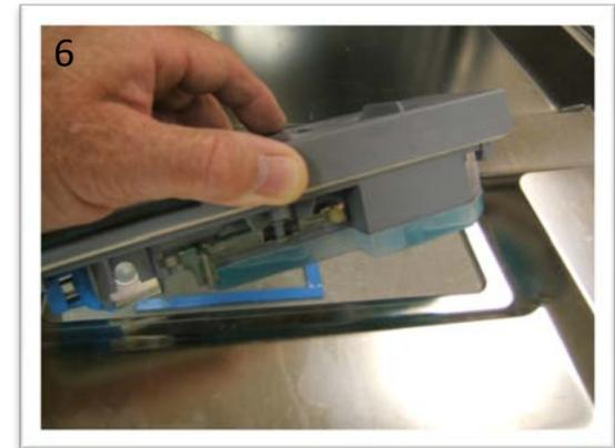
Open the door and lift assembly from inner door
