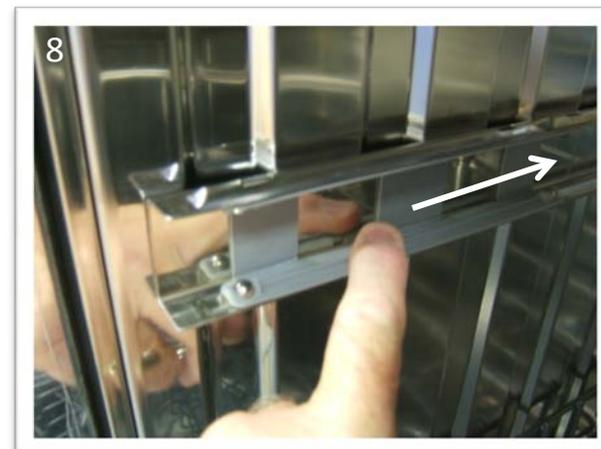
The replacement bearing holders come in a kit with the ball bearings. The bearing holder comes flat, insert the ball bearings into the holder, then bend the holder to form the correct shape (see illustration).
