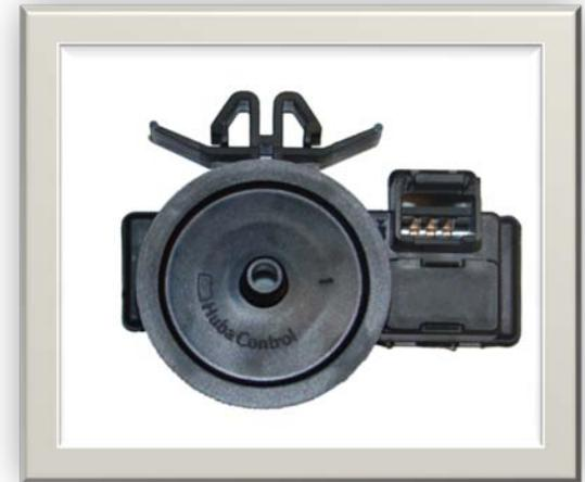
The pressure sensor is connected to the pressure chamber in the sump. It measures the pressure corresponding to the water level in the machine. In the event of an excessively high water level in the machine the drain pump starts and other components are switched off. When the right level is reached, the program will continue. If the level is not reached within one minute, the program stops and the machine will show a fault indication.
