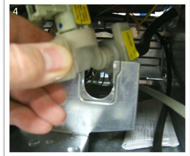
Slide the valve out of the bracket
