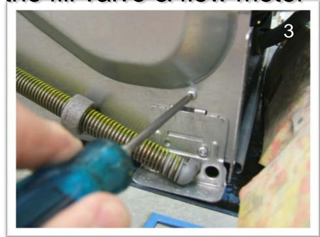
With a straight blade screwdriver rotate cover counter clockwise to remove. Remove single screw on outside and two from the inside of the tank.
