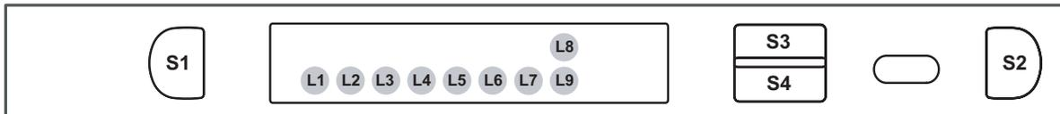
*L - LED, S - Push-button, F - Fault code on the display*
