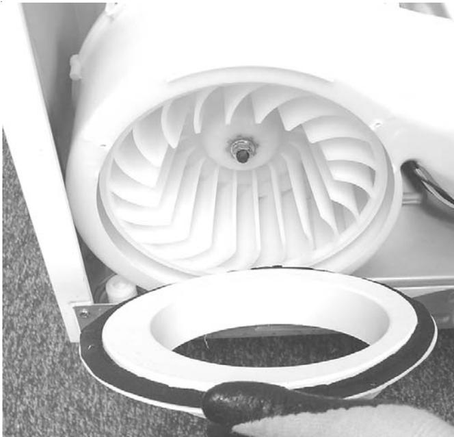
9. Removed the screw at the bottom of the blower housing.
