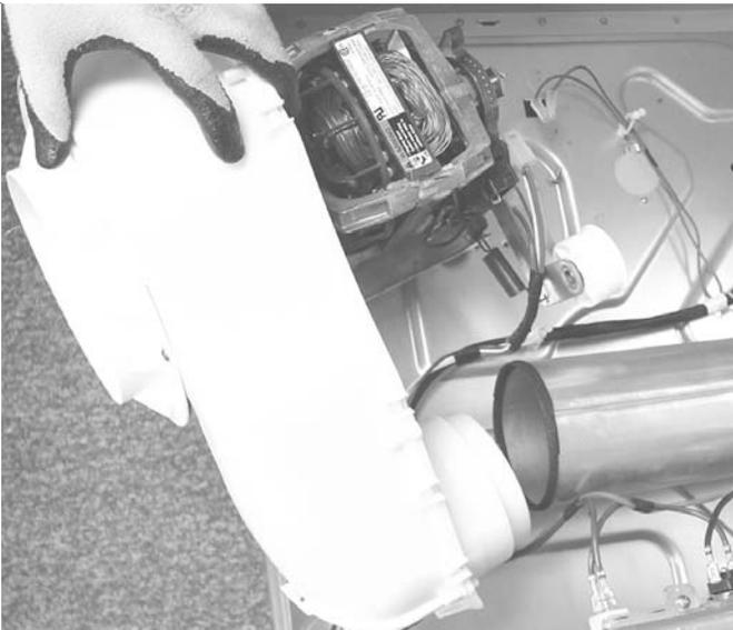
14. Remove the 14mm nut securing the blower wheel to the shaft. The nut is a left hand thread.
