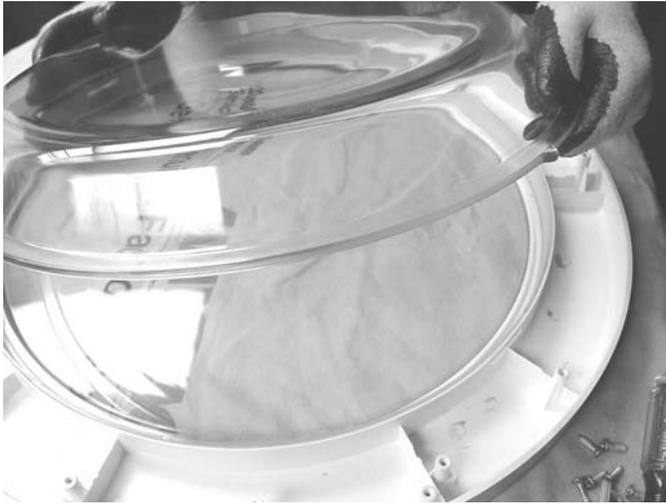
9. Remove outer door viewing panel. Insert screwdriver in slot to disengage latch.
