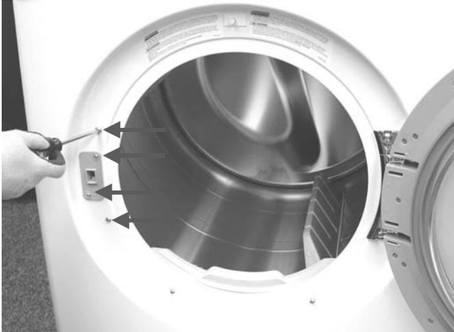
3. Remove two screws attaching Door Hinge.
