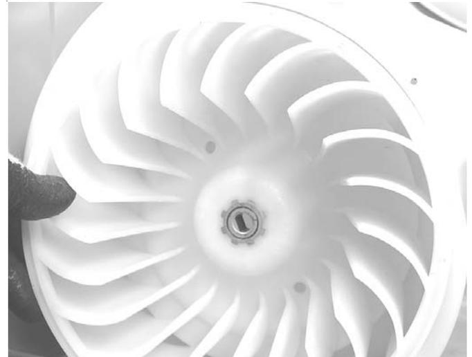
16. Remove the three screws securing the blower housing to the motor bracket.
