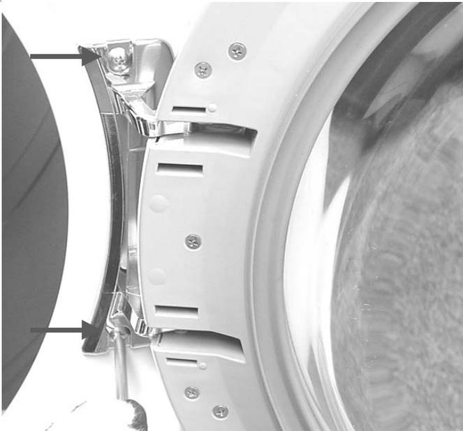
4. Install Door and Strike on opposite sides or continue with Door disassembly.
