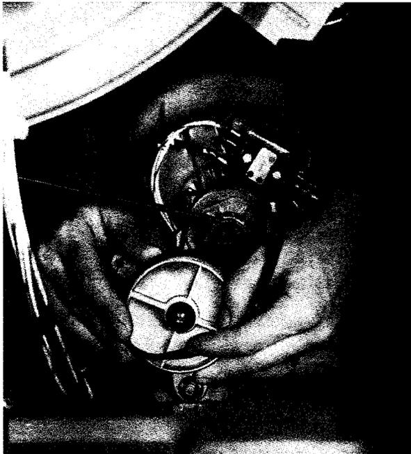
4. With the right hand, loop the belt over the top of the motor pulley making certain the grooves of the belt are against the pulley and that the belt is properly seated into the pulley.
