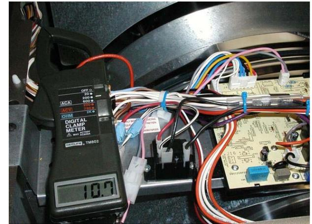
Check for heater current around orange wire to Triac MT1.
