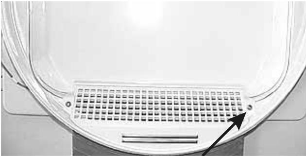
4. Pull the grill into the drum and disconnect the wires.
