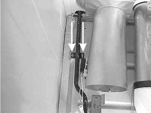
3. Remove the vent pipe out the rear of the dryer and remove the gasket from the vent pipe.
