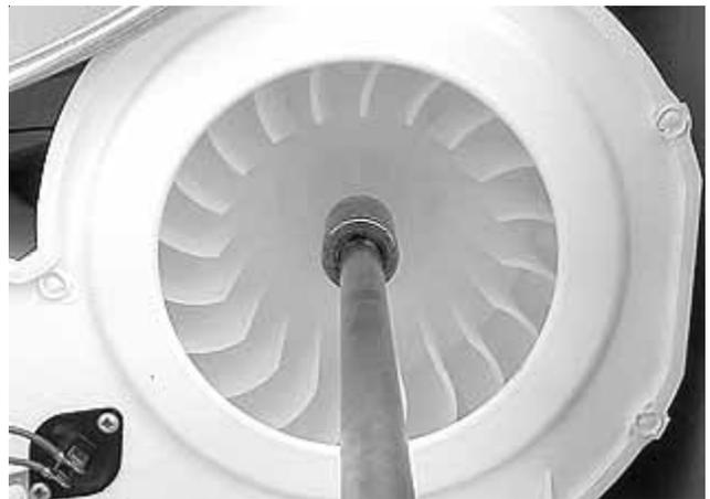
4. Remove (2) screws holding the housing to the dryer base.
