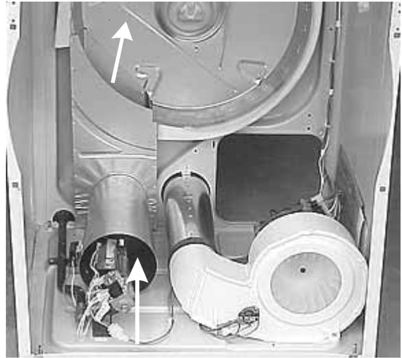
The drum is the same as in the electric dryer, except it does not have a heat baffle on it.
