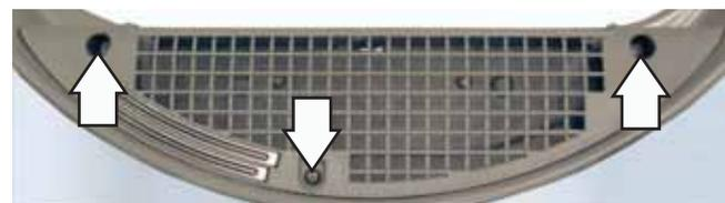
6. Remove the 2 Phillips-head screws that attach the filter guide and inlet to the drum support.
