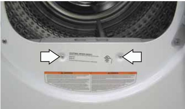
4. Close the door, then remove the 4 Phillips-head screws from the top corners of the front panel.
