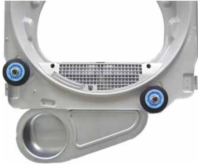
Each roller is part of an assembly that consists of a roller, roller shaft, 2 plastic triangular clips, 2 washers, and a 17-mm hex nut.
