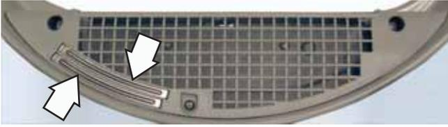
**Note:** The 2 touch sensors in the filter inlet are not replaceable. To replace the sensors, replace the filter inlet.
