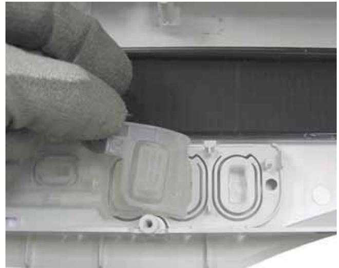
8. Release the 11 tabs that attach the button frame to the control panel, then lift the frame from the panel.
