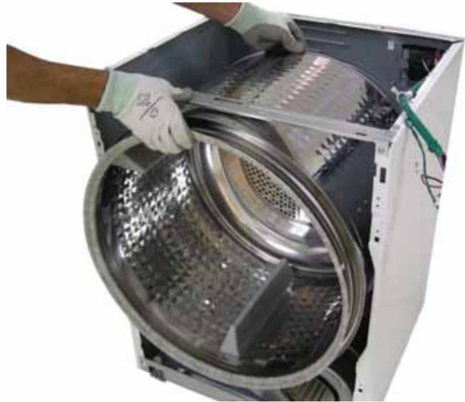
The drum shaft is permanently attached to the back of the drum. A plastic washer is installed on the drum shaft.
