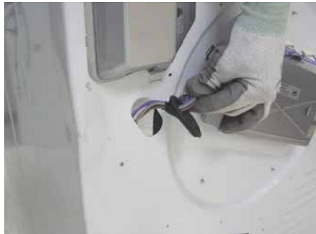
7. Remove the 2 Phillips-head screws that attach the heater assembly to the back of the cabinet.
