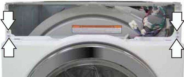
5. Pull the top of the front panel away from the cabinet, then disconnect the door switch wire harness.
