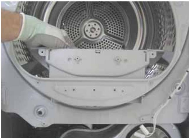
**Note:** The filter guide is attached to the filter inlet with 2 tabs, 1 on each side.
