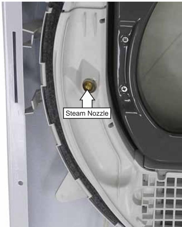
The steam nozzle can be replaced without disassembly of the dryer. Replacement can be performed by opening the dryer door to access the steam nozzle. A 7/16" or 11-mm nut driver can be used to unscrew the nozzle from the air duct assembly.
