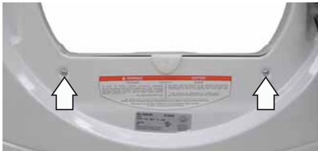
4. Grasp each side of the air duct assembly and unsnap the air duct from the front panel.
