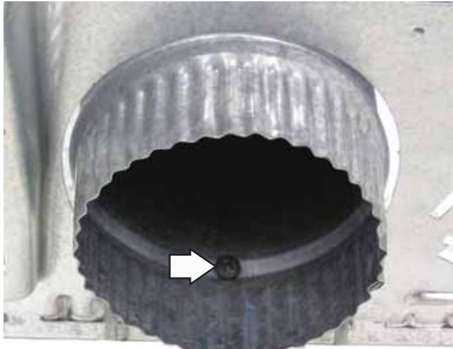
3. Remove the 7 Phillips-head screws that attach the blower housing to the base plate.
