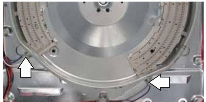
3. Bend back the single metal tab on the housing holding the heater in place.
