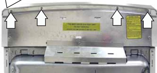
3. Rotate the control panel forward approximately 1 inch, then slide it to the right to unlock the 3 bottom lock tabs.
