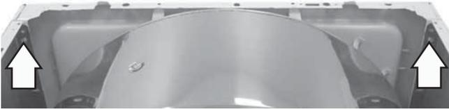
3. Tilt the top edge of the front panel out and disconnect wiring to the door switch, light, and sensor rods.
