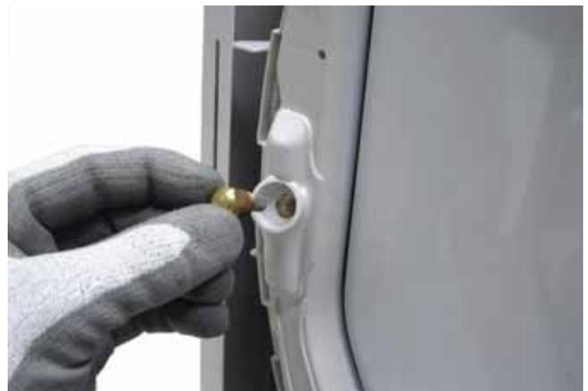
**Note:** The replacement steam nozzle will have thread lock pre-applied to the screw threads.
