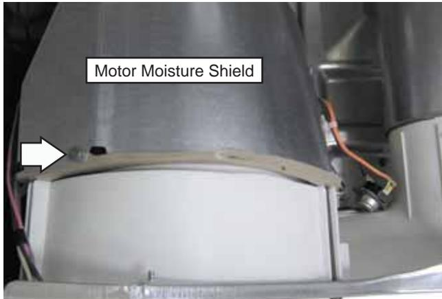
6. Invert the motor moisture shield, then compress and remove the wire tie from the shield.
