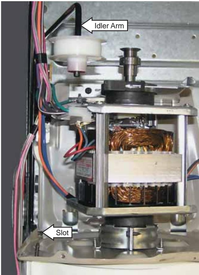
4. Remove the idler assembly from the dryer.
