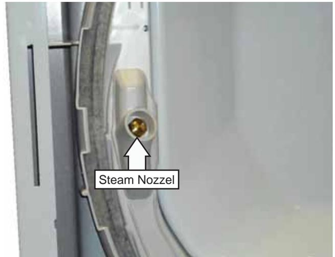
The steam nozzle can be replaced without disassembly of the dryer. Replacement can be performed by opening the dryer door to access the steam nozzle. A 7/16" or 11-mm nut driver can be used to unscrew the nozzle from the air duct assembly.
