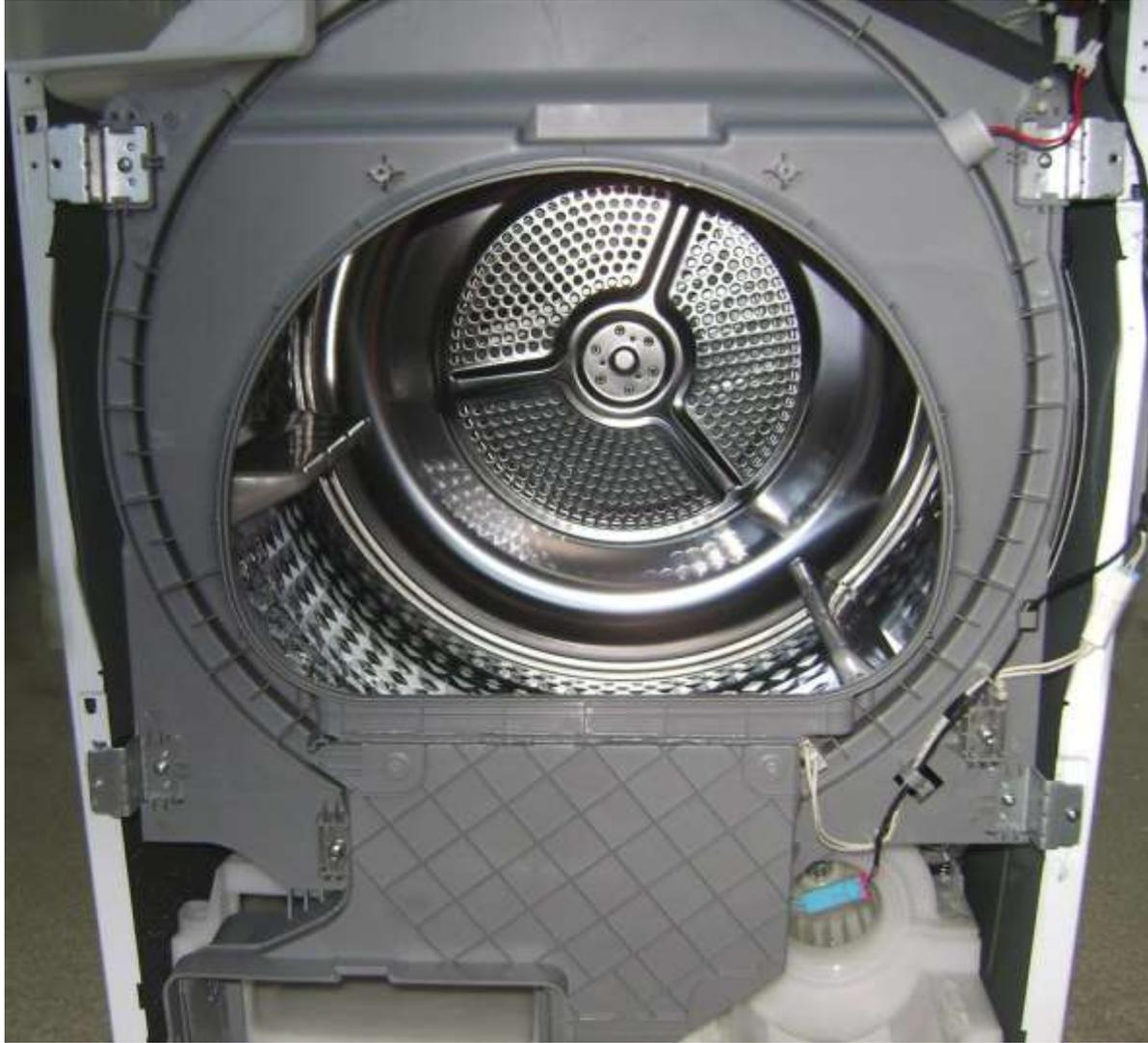
**Remove towel and finish installation of front frame. Test belt for fit**
