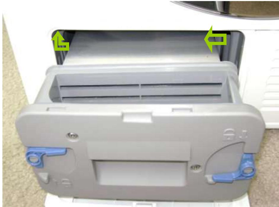
**Condenser pulled slightly forward to view “ambient” air flow pattern**
