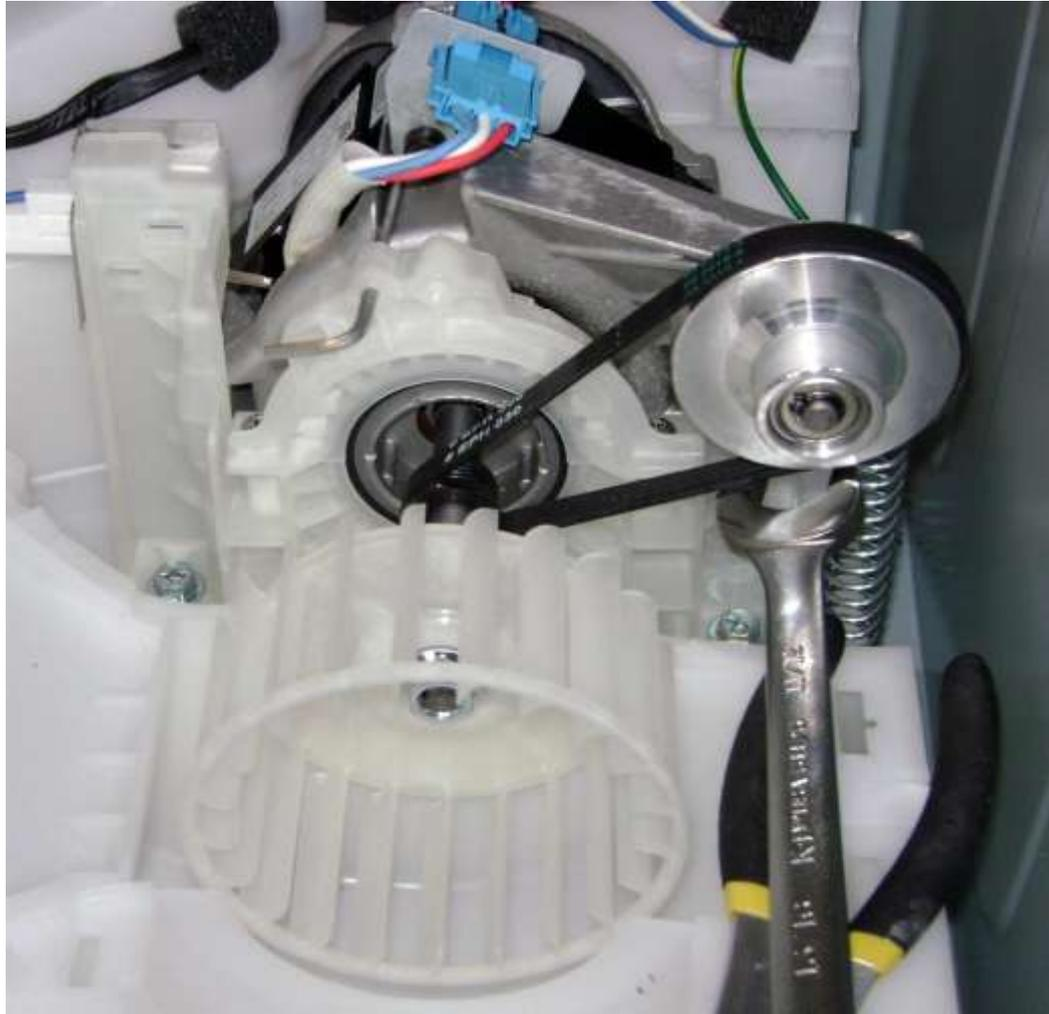
**If unable to lift motor by hand to insert support tool, technician would need to pry up on motor pulley in some manner. Care should be taken to not damage drive belt**
