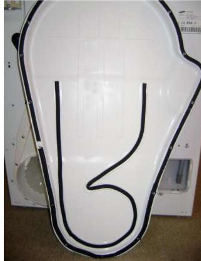
**Duct cover removed and turned around to view sealed area for air.**
