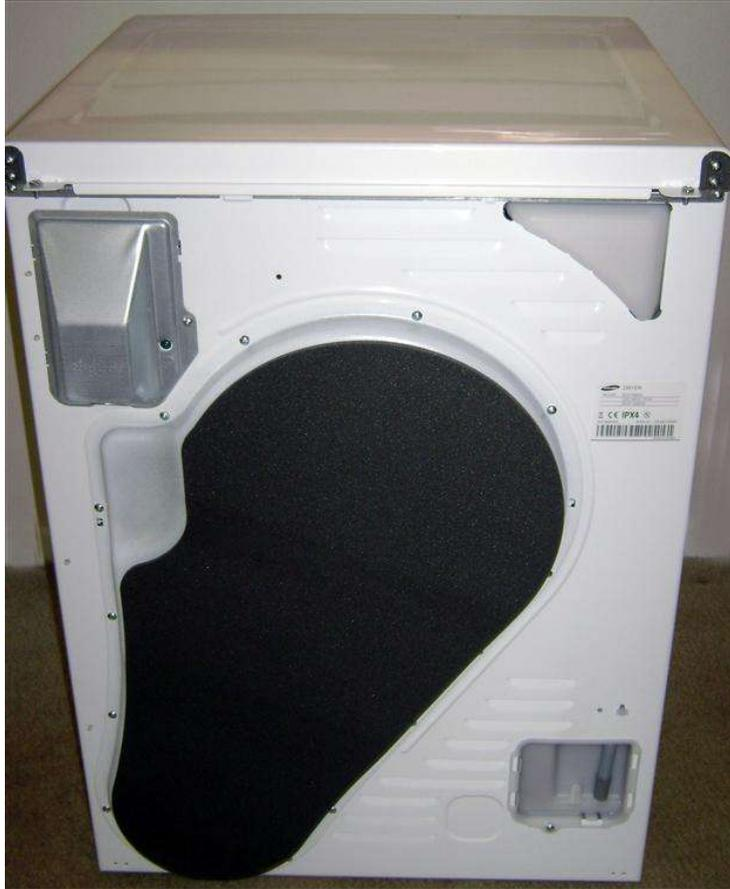
**View of dryer from rear with rear duct cover in place.**
