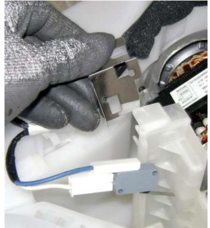
**Removed with tabs on housing**
