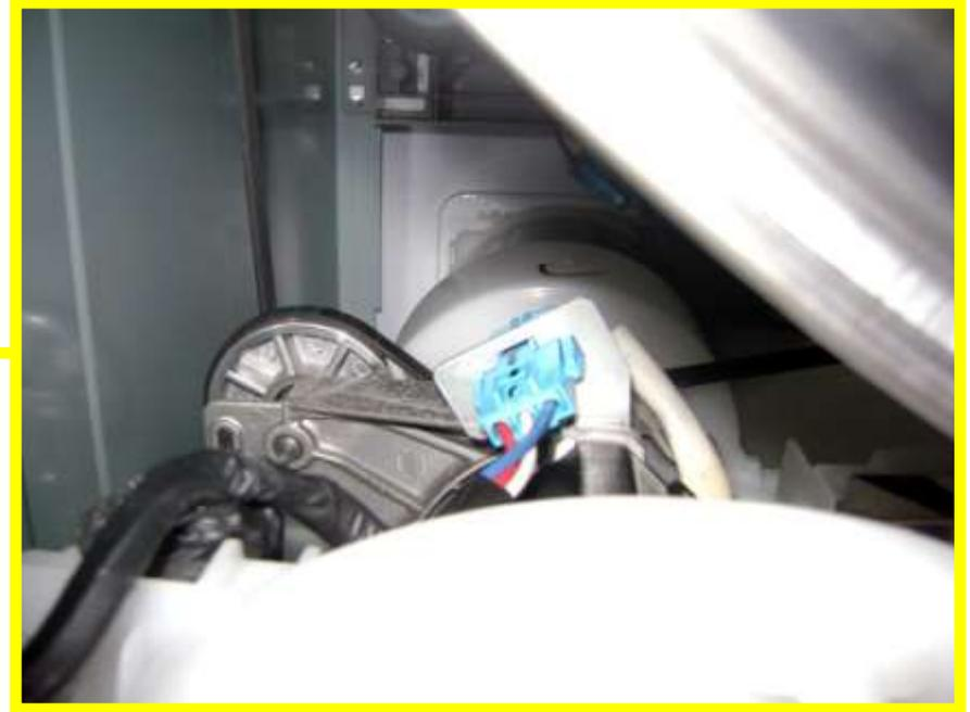
**Rear view of motor connections and drum belt**
