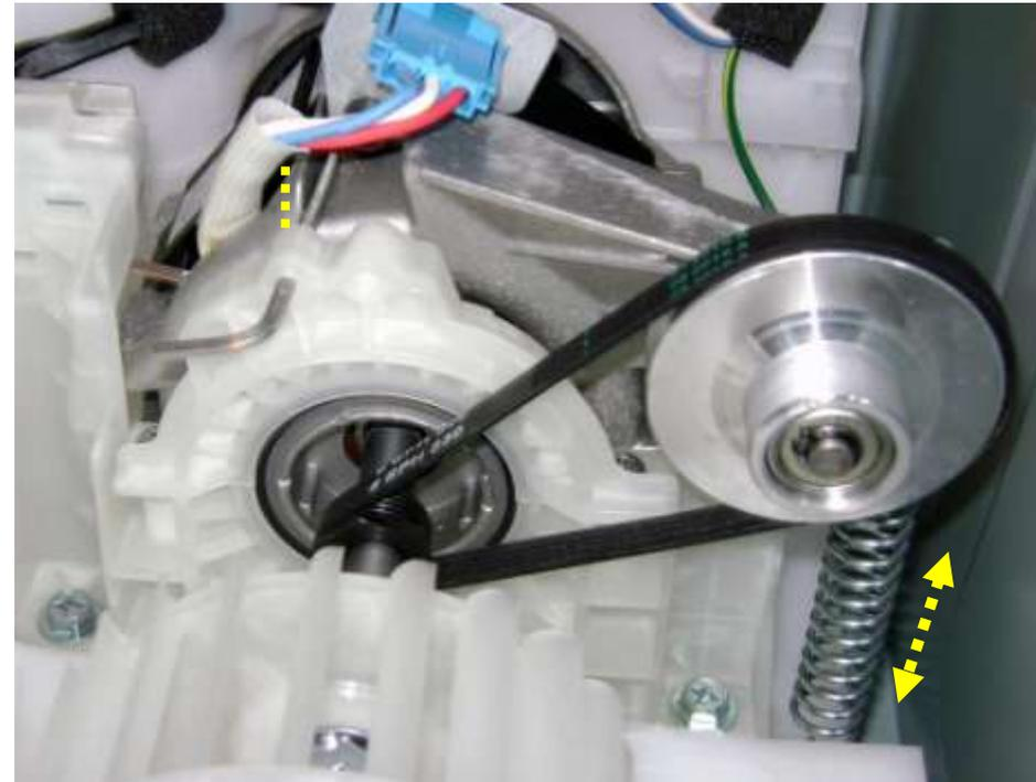
1/8 allen wrench or other similar size tool will fit in the hole and used notched area of motor to take up spring tension.
