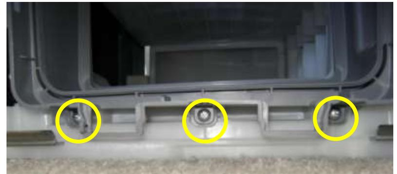
**Remove 3 screws located below condenser**
