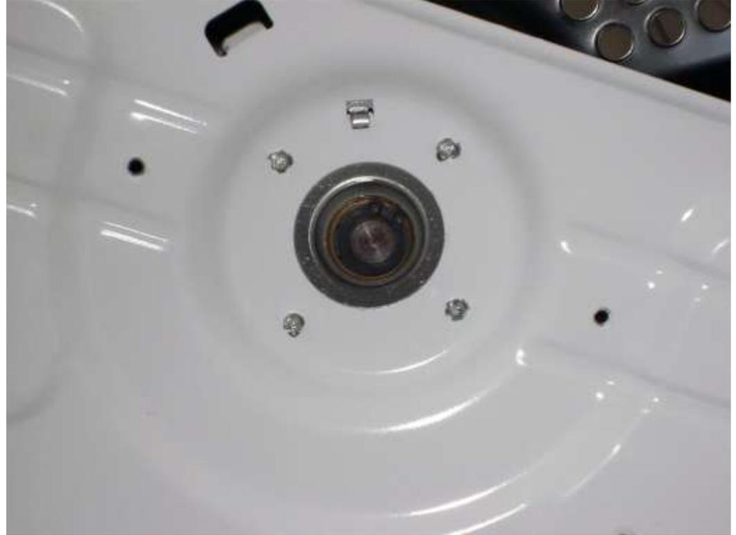
**Remove C-clip securing drum shaft**
