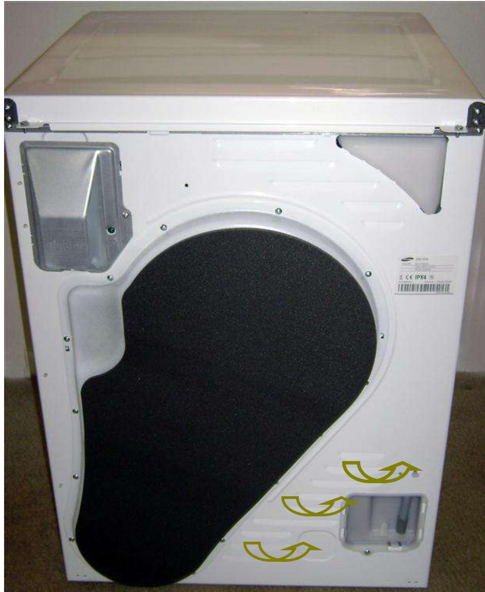
**Heated ambient air exits rear of machine**
