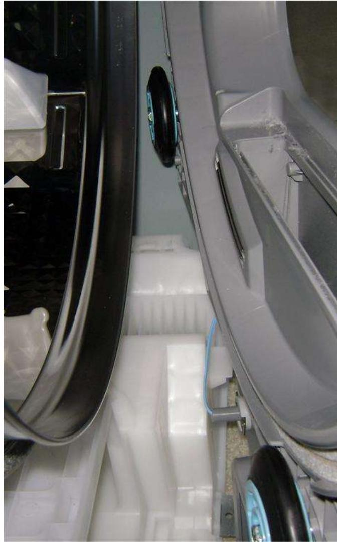
**Install front frame.. lower section first to line up drum and rollers**
