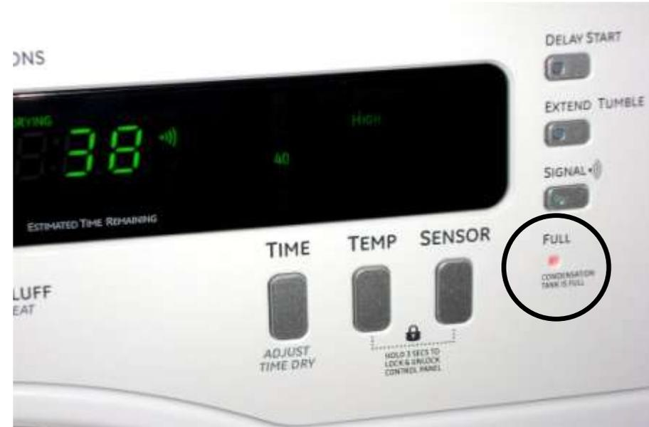
Pump runs to try and pump excess water out of sump. Eventually it could pause cycle and light the **red** “Full” LED as shown in picture.
