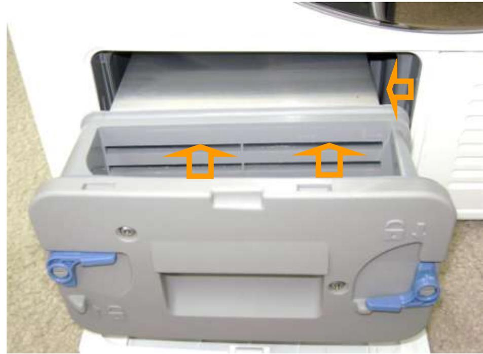
**Condenser pulled slightly forward to view “process” air flow pattern**
