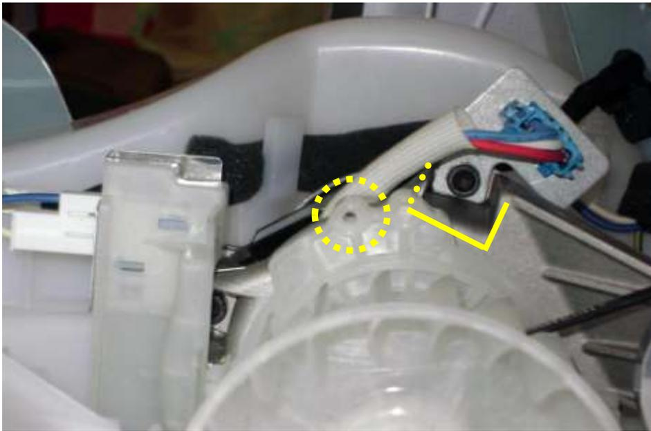
Note hole in top motor support bracket as well as “notched” area of motor housing
