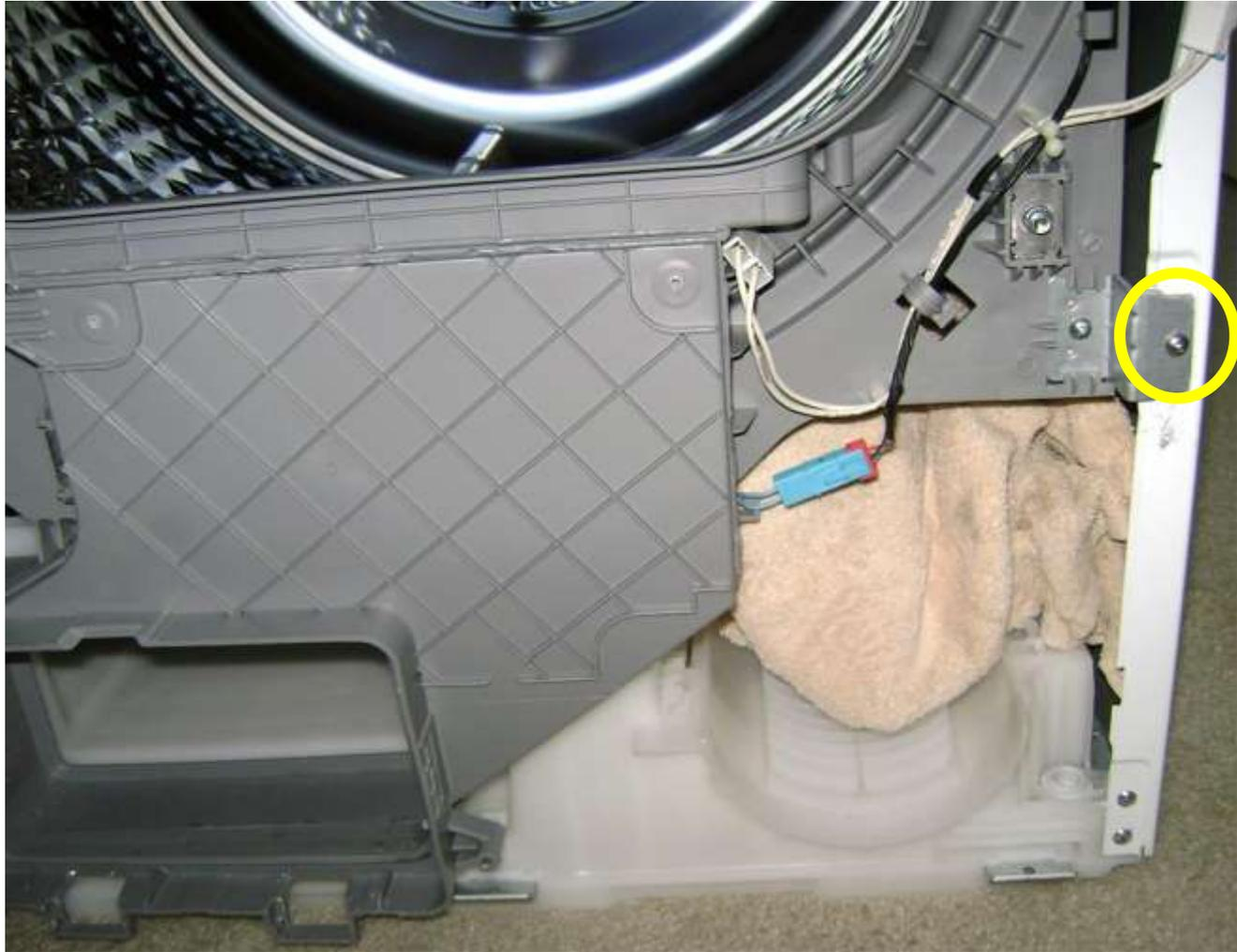
**Install lower right side screw first for support of front frame, and then other screws, while noting position of drum lip and belt.**
