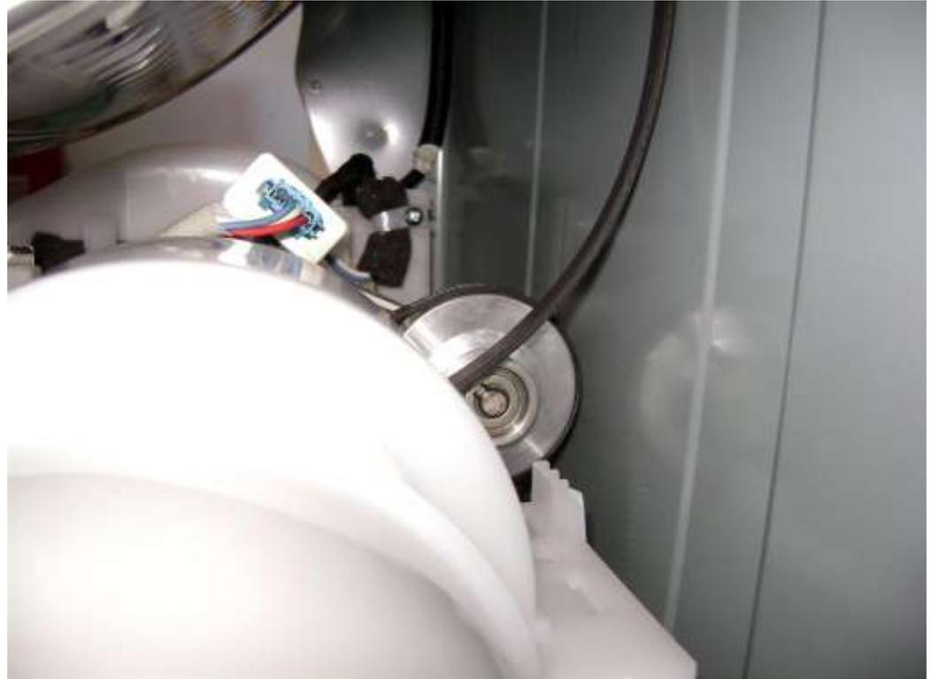
**Remove front panel to gain access to the drum belt.
