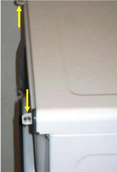
**Remove two 10mm/Phillips screws in the back.**
