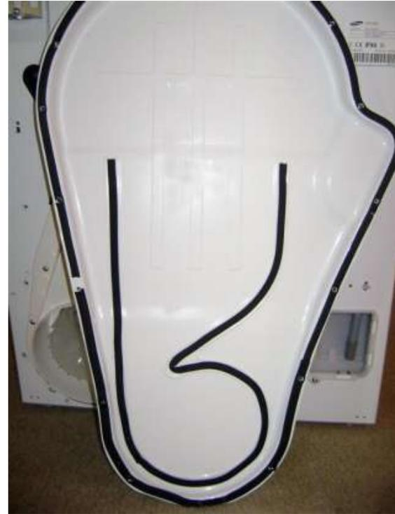
**Duct cover turned around to view air seal**
