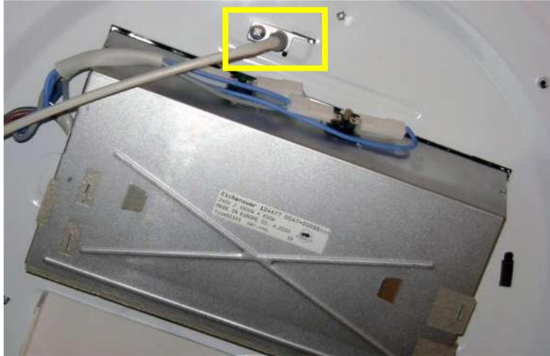
**Inlet thermistor located above heater and replaced with single screw 49K @ 77F**
