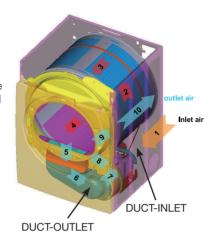
Any air leaks between air inlet and the blower such as drum front felt or cover duct to cabinet front sealing will result in improper temperatures. The air being pulled down the cover duct to the drum outlet thermostat will be cooler than normal, giving this thermostat a false indication (delayed or no trip).
