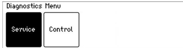
Press and hold the **WRINKLE FREE** button and then press the **SELECT** button. Keep the buttons pressed for at least 2 seconds, after which time two beeps will sound and the screen above will appear. Press the **SELECT** button again to enter the service screen.
