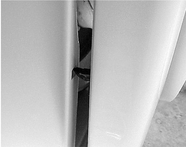
5. Lift up on the front panel to release the (2) tabs at the top, one on each end, and swing the panel out.
