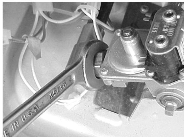
5. Remove the (2) screws holding the manifold pipe to the base and lift the pipe out.
