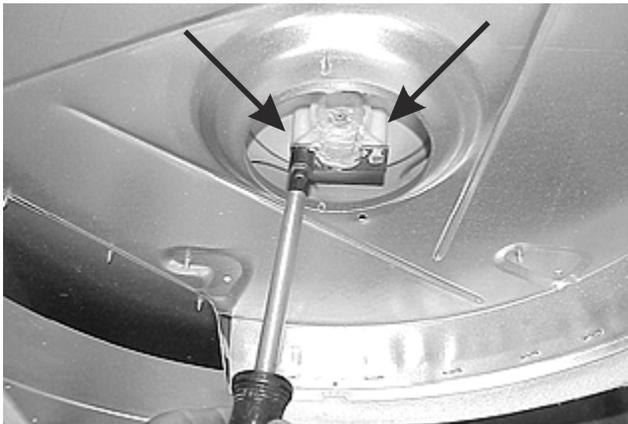
**Note:** Do not lose the grounding ball or the tinnerman mounting clip from the rear of the dryer.
