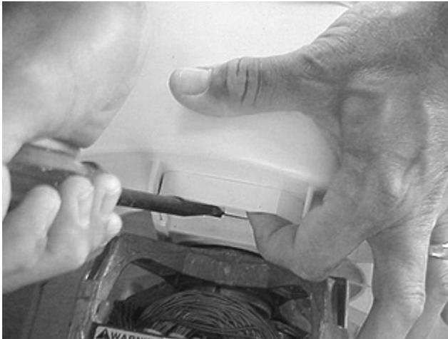
6. Raise the front of the motor and pull the housing forward.
