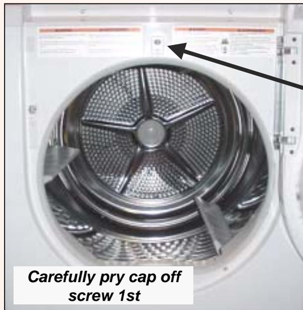
**HINT:** If the dryer won't operate, check to see if the door switch is being activated by the door pin.
