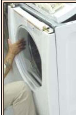
**HINT:** When aligning front panel tabs on frame, make sure door seal is seated properly.
