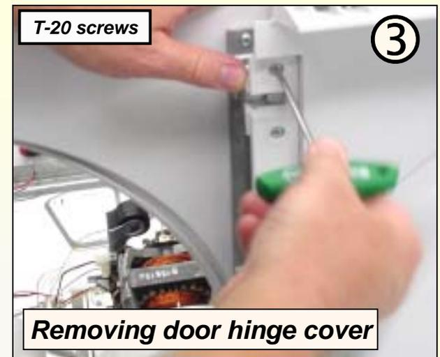
*Rear access is best for most repairs.*
