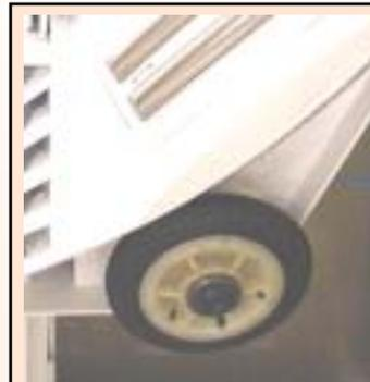
**HINT:** Reconnect drum belt after front panel installation so drum (& support wheels) won't be in tension. After belt installation, reset broken belt switch.
