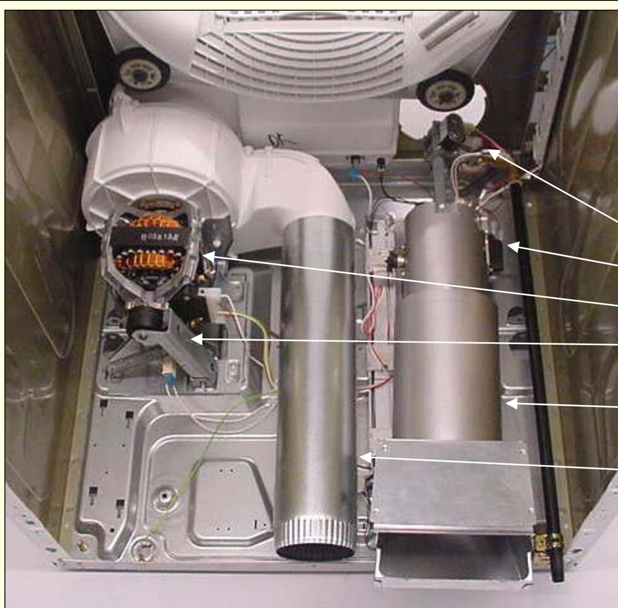
*Gas dryer after drum has been removed.*
