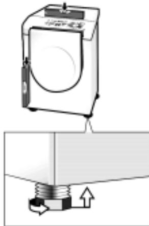
The dryer should be level with all four feet firmly on the ground. The dryer must not wobble. If the dryer is not level or if it does wobble, the feet must be adjusted. Adjust the height-adjustable feet until the dryer does not rock and is level, both front-to-back and side-to-side.
