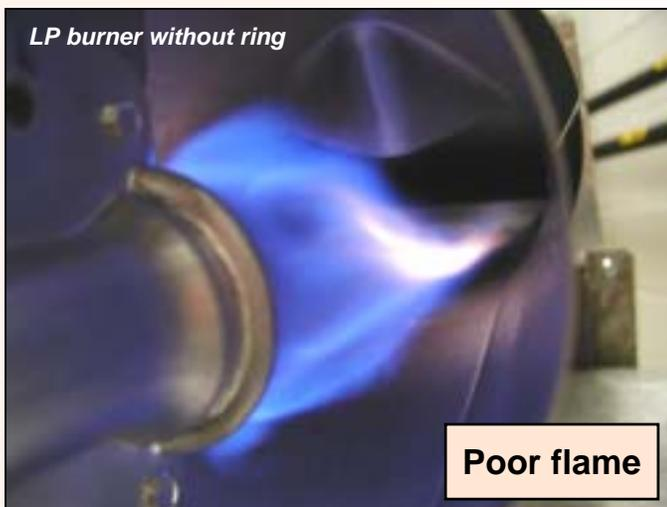
**Poor flame** – poor air flow through burner (from blocked burner air holes) causes a lazy, long and quiet flame with some yellow.
