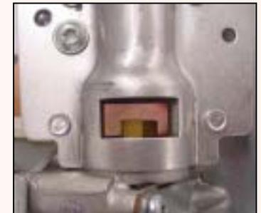
For best results, fan must be running and burner air holes must be clear.
