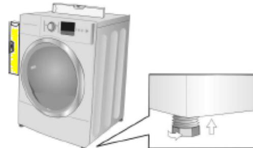
To adjust feet (leveling legs), rotate left to right to lower dryer.
