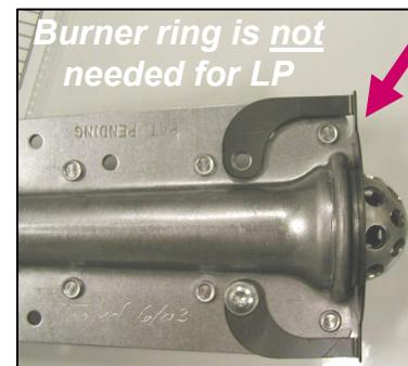
Remove the burner ring since it's not needed for LP.
