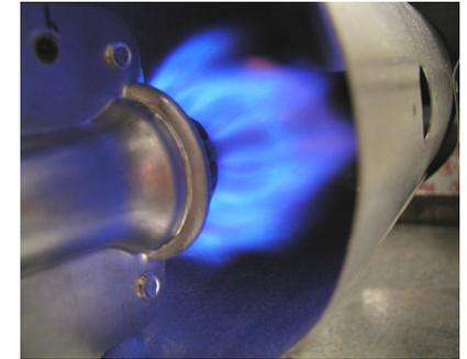
The gas dryer burner circuit runs through the motor & Hi-limit. The connection through the motor cuts out the burner if the motor isn't running.
