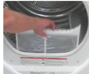
If the *Filter* light won't turn off, clean the lint filter (by hand) with dish soap and water. The lint filter is very fine and can be clogged over time when fabric softener or softener sheets are used.
