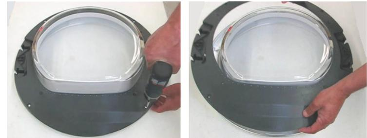
The door glass bowl is shown here in the standard hinge right position. Note the door glass and inner ring positions before removing them as they change depending on the hinge position (right or left).
