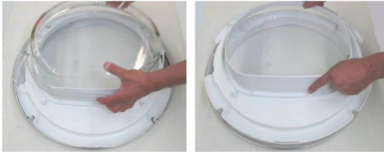
Lift the outer door glass cover from the outer door frame.
