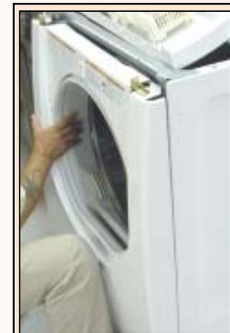
**HINT:** When aligning front panel tabs on frame, make sure door seal is seated properly.
