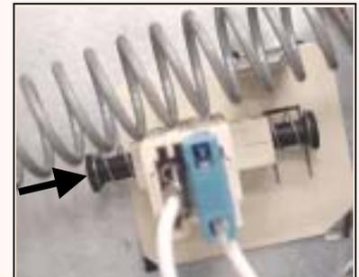
**HINT:** To reset the broken belt switch, push in the left black plunger (viewing rear of motor).
