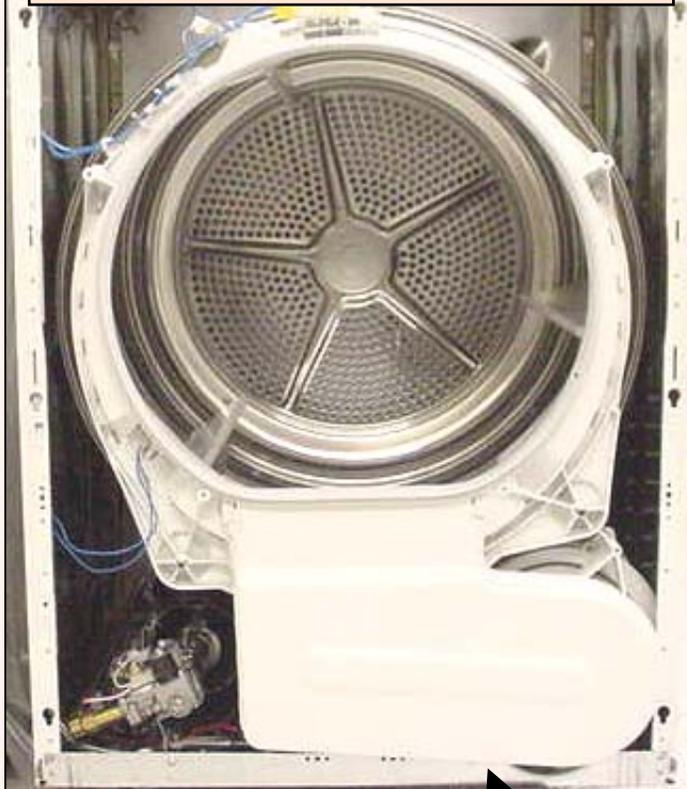
**HINT:** When installing front shield, make sure notch on bottom is seated on frame.
