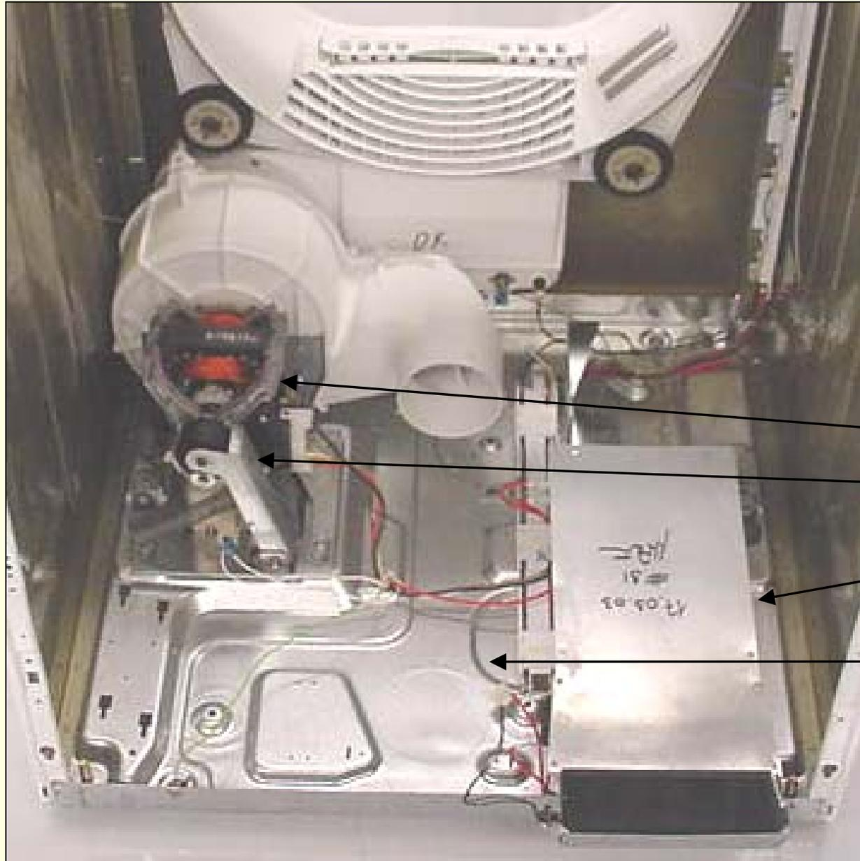
*Electric dryer after drum has been removed.*
