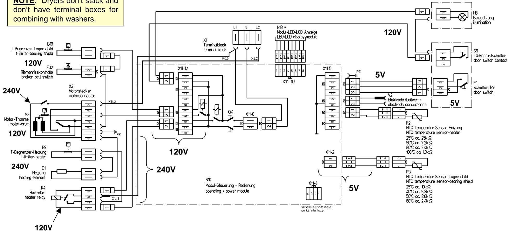
**NOTE:** Motor cutout switch cuts out the heater if the motor shuts down.
