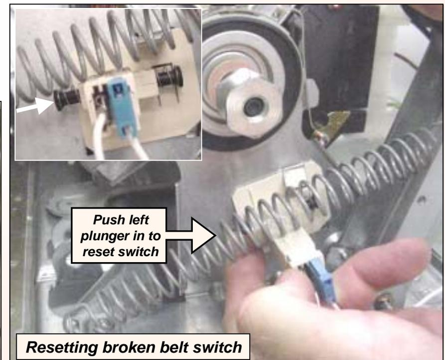
Push left plunger in to reset switch
