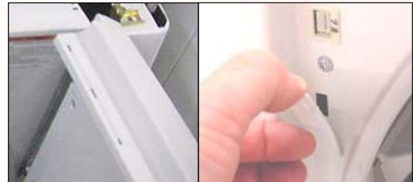
**HINT:** Kit includes instructions & all parts, including red & white strips for door (showing door “handle” location) & covers for unused openings. Remove red & white strips (to exchange positions) by squeezing them from behind.
