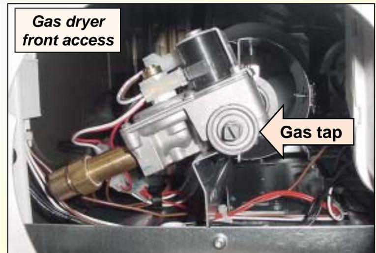
**HINT:** Gas valves and burners are attached together to a single bracket. To remove them, screws must be removed from the base and burner chamber.
