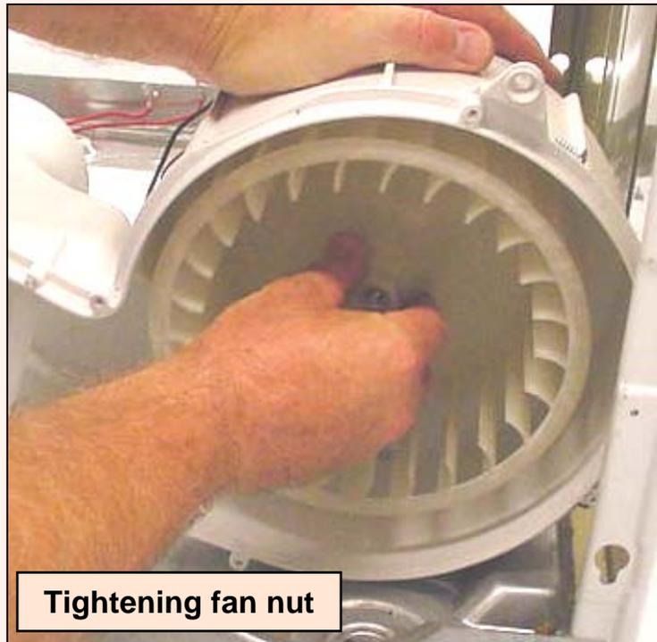
**HINT:** Make sure fan is tight. If fan nut won't tighten down adequately, install a lockwasher.
