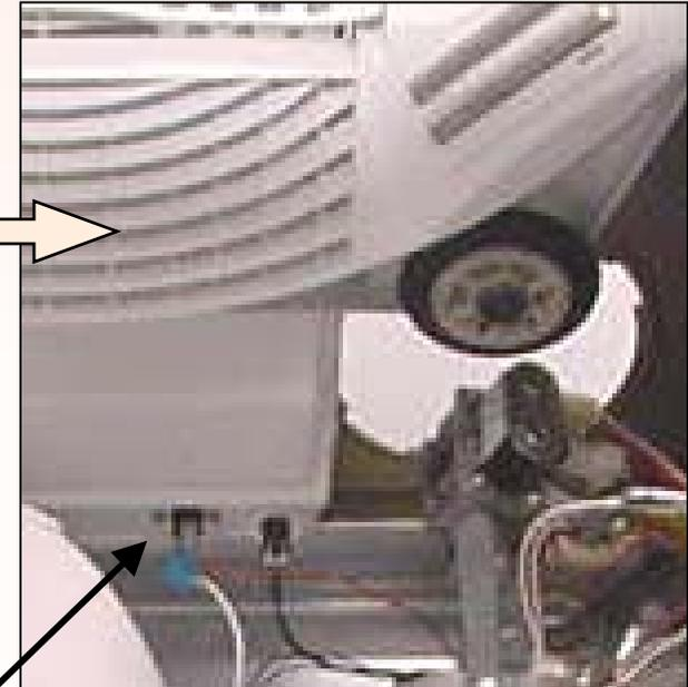
**NOTE:** Fault codes E:01, E:11 & E:12 occur when lint screens are clogged. Control module reads NTC and approximates air flow – when air flow is too low, fault codes are generated. B19 Hi-limits do not generate fault codes.
