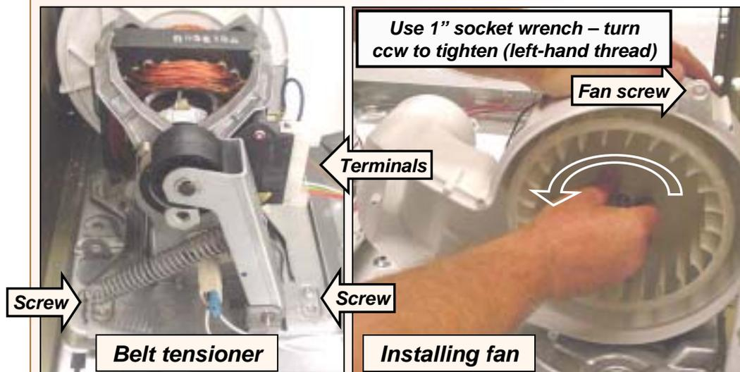
Use 1" socket wrench – turn ccw to tighten (left-hand thread)
