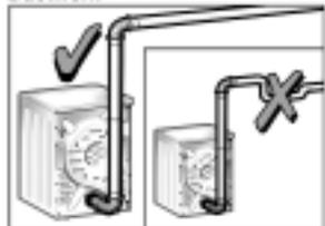
To ensure optimum performance, the ducting system of the dryer should be as short as possible with a minimum number of elbows. Your dryer will work best when the venting system has as few air flow restrictions as possible. Exhaust ducting which is longer than recommended may extend drying time, cause lint to accumulate and affect dryer performance and dryer life-time.
