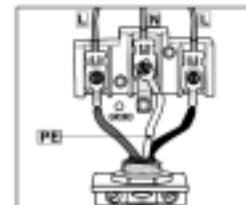
7. Tighten the screws (2.5 Nm) on the U.L. strain relief clamp so that the power cord cannot be moved.
