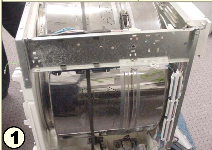
Frame with fascia, front & side panels removed.
