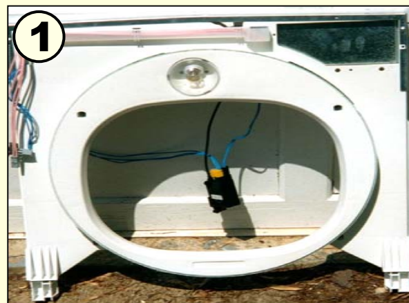
Frame with fascia, front & side panels removed.
