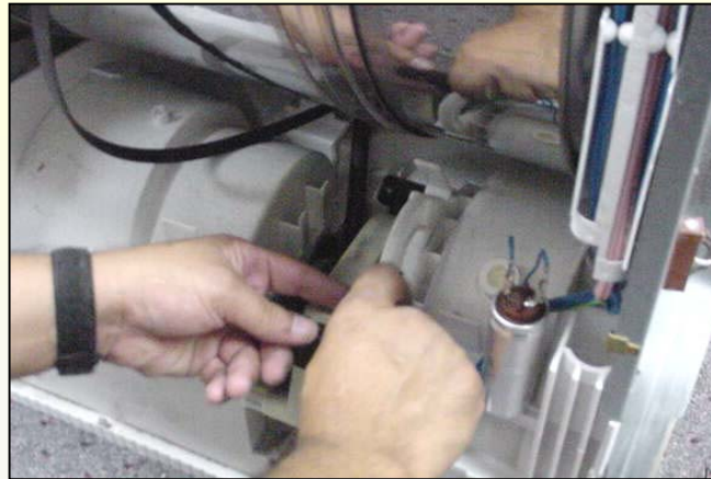
Slide drive belt off pulley
