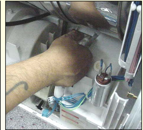
Pull out motor clamp
