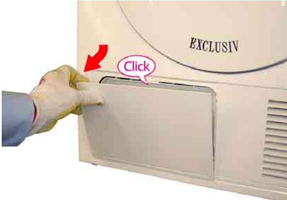
Removing the cooling-air panel
