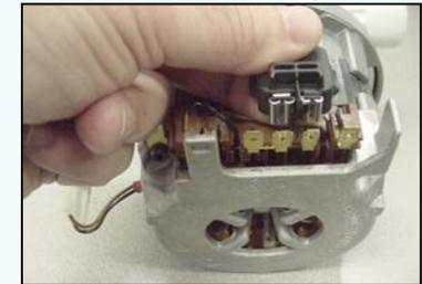
To install (PTC) motor starters, push female terminals over pump motor terminals 2 & 4. The terminals are different sizes to match the smaller motor terminal 4.
