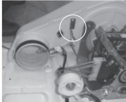
2. Separation of thermostat fan: Separate connector. → Remove 2 screws.
