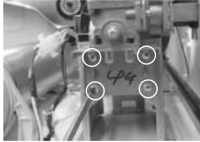
2. Remove 1 screws at the back of cabinet.
