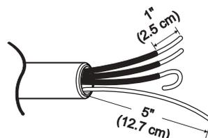
Then, put the hooked shape end of the wire under the screw of the terminal block (hooked end facing to the right) and pinch the hook together and screw tightly.
