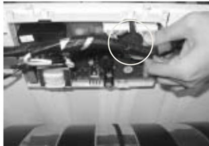
3. Separate humidity sensor connector.
