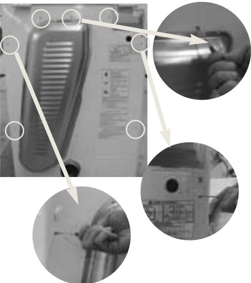
3. Remove support drum rear ass'y in the direction of →
