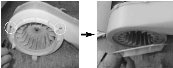
3. Separation of impeller fan: Fix motor axis and separate fan.
