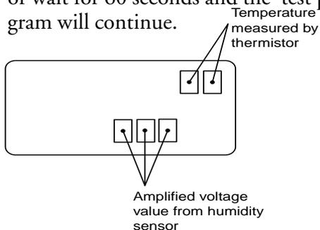
The program heats, increasing the temperature by 14° in max. 10 minutes, then allows it to cool for 5 minutes (testing that the heating element is working).
